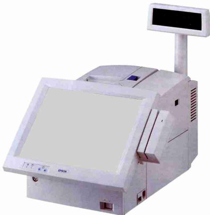
Figure 8 Epson IM-310 incorporating DM-D106 customer display and TM-88II printer
