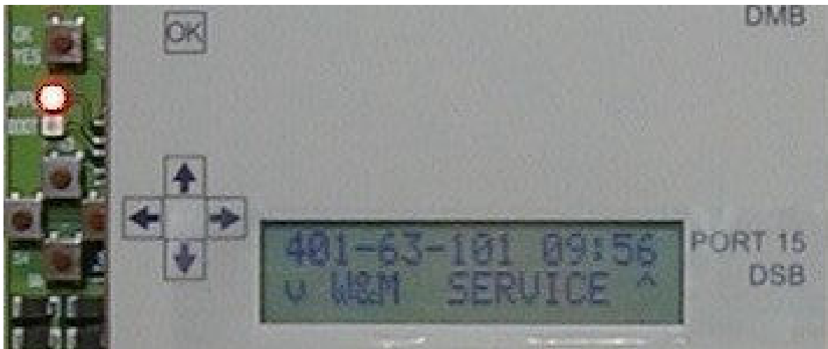
Figure 4 Central Processing Board (CPB508) display and menu navigation keys
