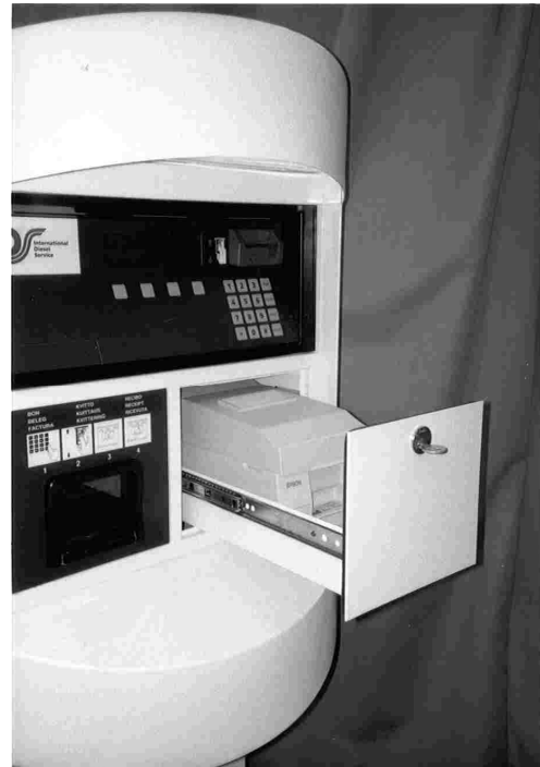
Figure 4 Views showing printer access LH view: receipt printer RH view: journal log printer
