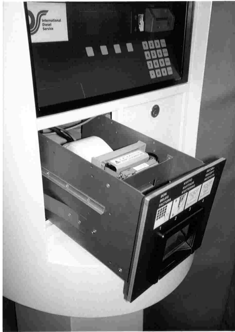
Figure 4 Views showing printer access LH view: receipt printer RH view: journal log printer
