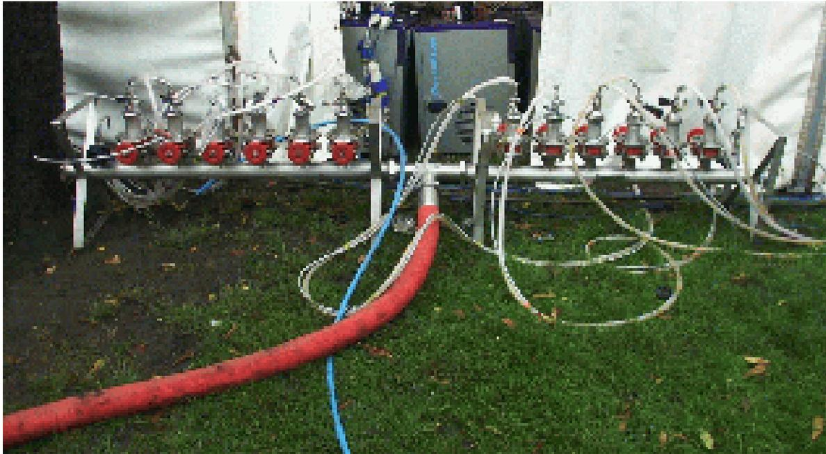
**Figure 6 Road Tanker Manifold and coupling devices**
