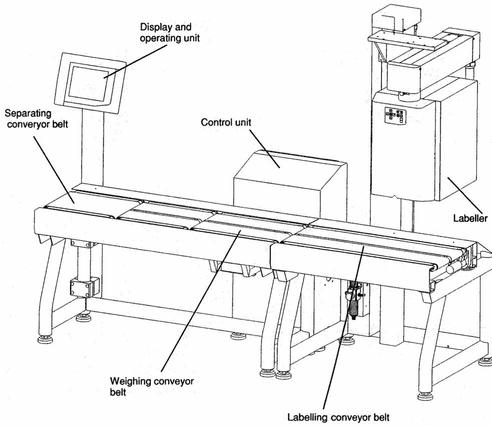
**Figure 1 Schematic of GLM-I system**
