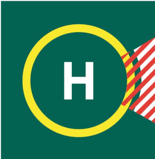
Figure 5 - Example of Prohibited Landing Heading Marking
