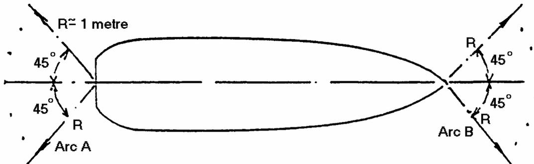
The "near the model" wave measuring probe to be positioned either on arc A or arc B
