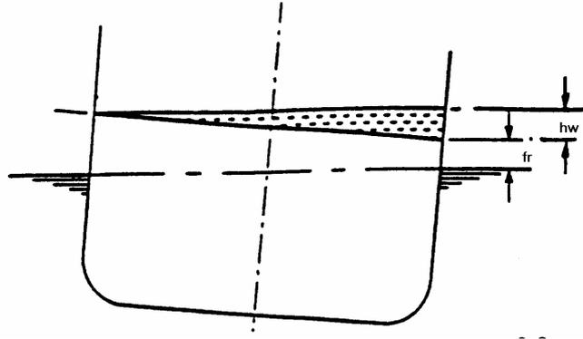
1. If  $f_r \geq 2.0$  metres, height of water on deck ( $h_w$ ) = 0.0 metres
