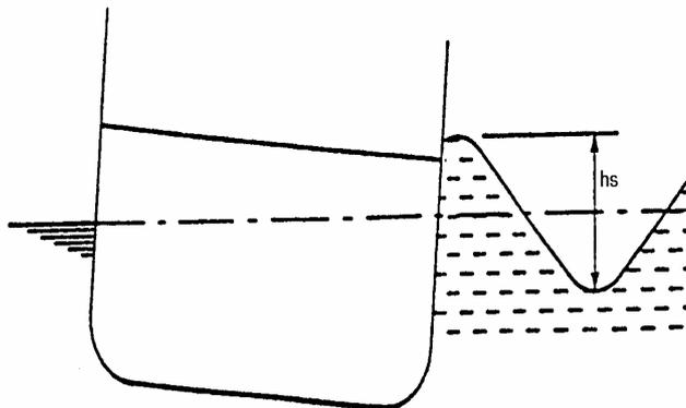
1. If  $h_s \geq 4.0$  metres, height of water on deck is calculated as per figure 3
