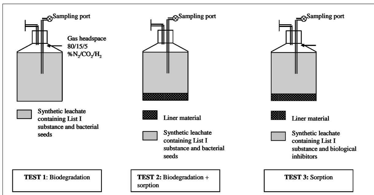
**Figure 6.1 Experimental set-up of the biodegradation tests using synthetic leachates**
