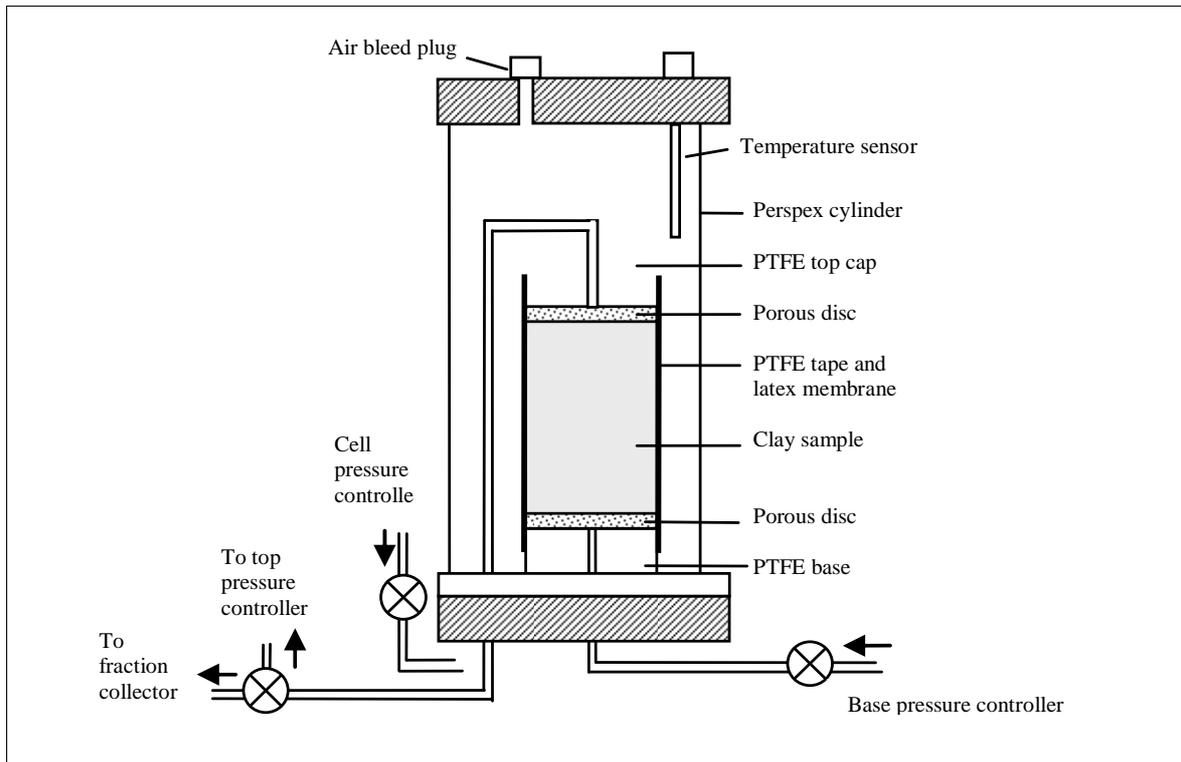
**Figure 5.1 Triaxial cell used in the column tests**
