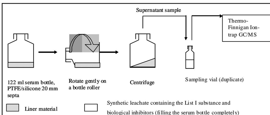
**Figure 3.2** Experimental set-up of the sorption batch tests
