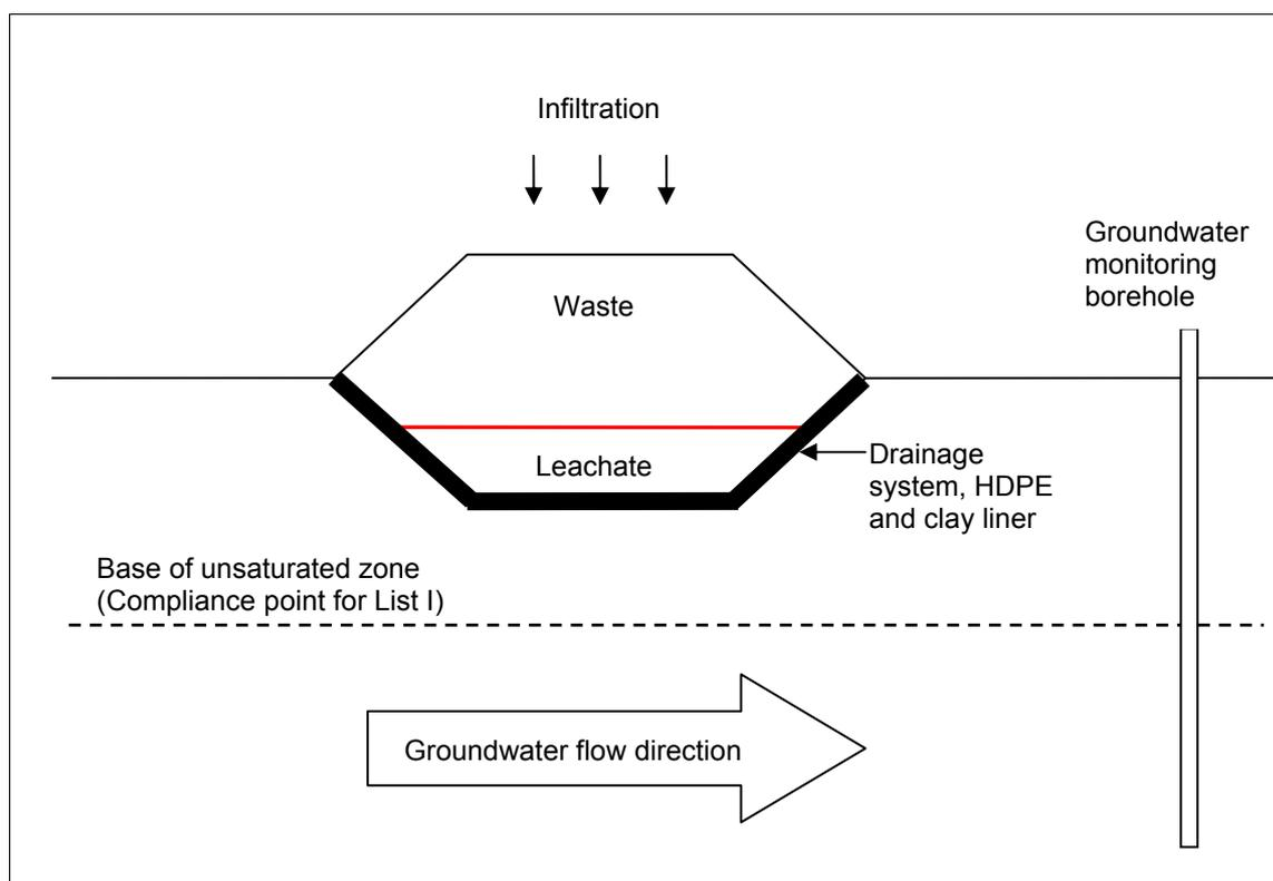
**Figure 7.1 Conceptual model for LandSim simulations**
