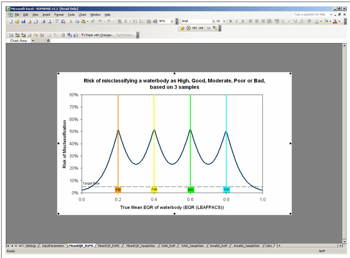
**Figure 3.3 MeanEQR\_RoM1 worksheet showing the risk of misclassifying a water body as High, Good, Moderate, Poor or Bad.**
