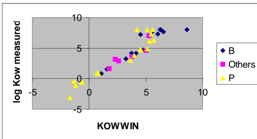
**Figure A4.1: Correlation between measured  $\log K_{ow}$  and that predicted by KOWWIN.**
