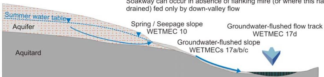
Figure 6.42 Schematic sections of types of Seepage Flow Tracks (WETMEC 15)
