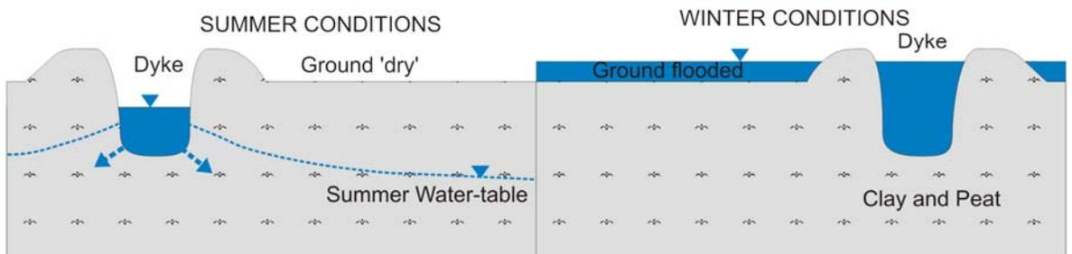
**Figure 6.16 Schematic sections of Summer-Dry Floodplains (WETMEC 5)**
