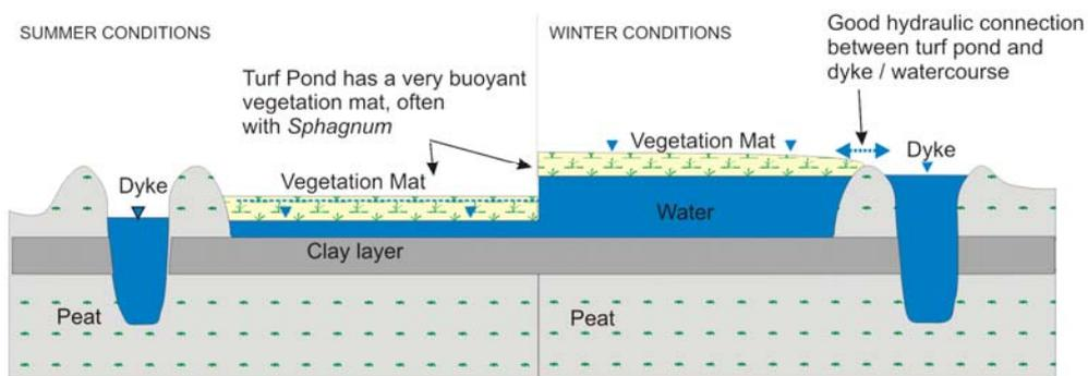
Figure 6.21 Schematic sections of Surface Water Percolation Floodplains (WETMEC 6)
