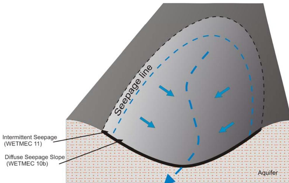
(B) Valleyhead trough with the Seepage Percolation and Soakway components absent or poorly developed (e.g. Scarning Fen). Some of these valleyheads *may* represent former examples of Seepage Percolation Troughs (a), which have been drained and stripped of much of their peat infill.
