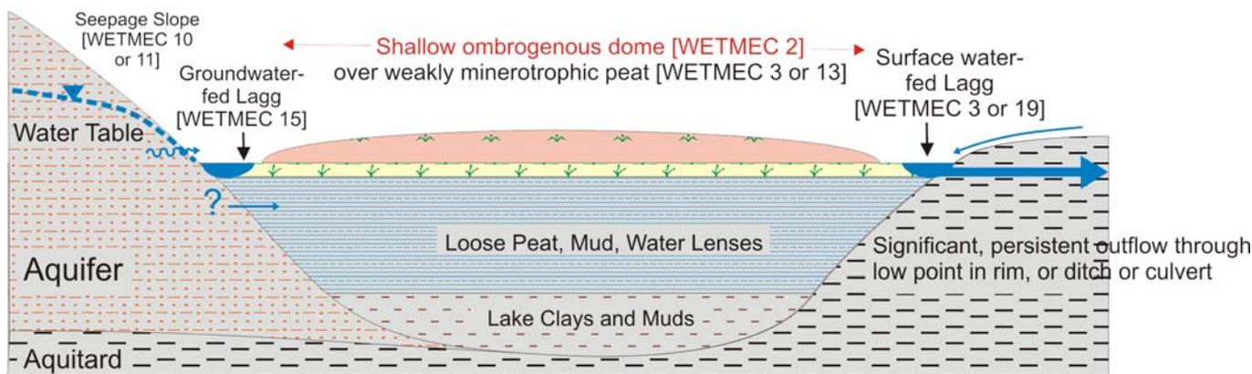
Figure 6.9 Schematic sections of Buoyant Ombrogenous Surfaces (WETMEC 2)
