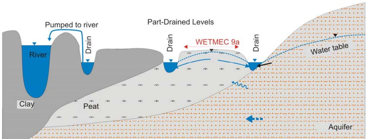
Figure 6.29 Schematic sections of Groundwater-Fed Bottoms (WETMEC 9)
