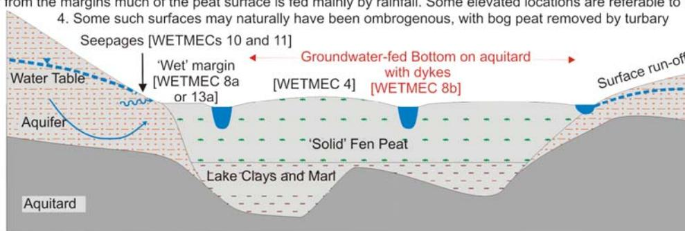
Figure 6.26 Schematic sections of Groundwater-Fed Bottoms with Aquitard (WETMEC 8)
