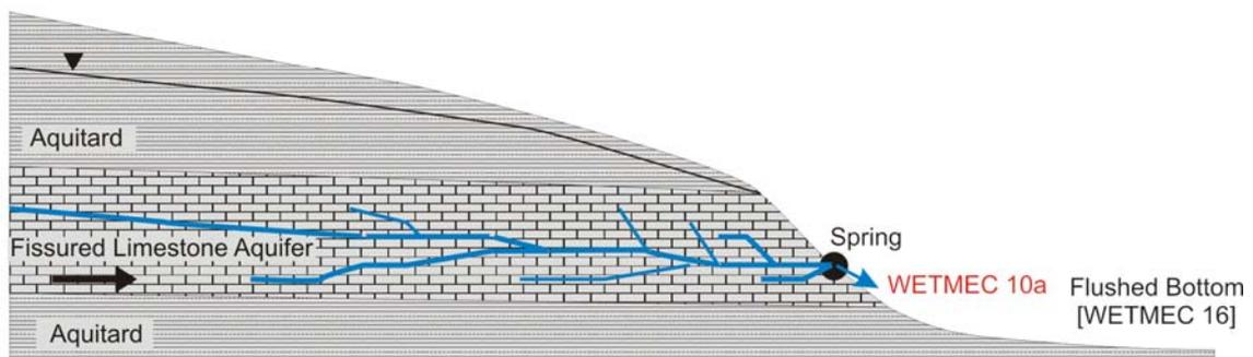
**Figure 6.31 Schematic sections of types of Permanent Seepage Slopes (WETMEC 10)**
