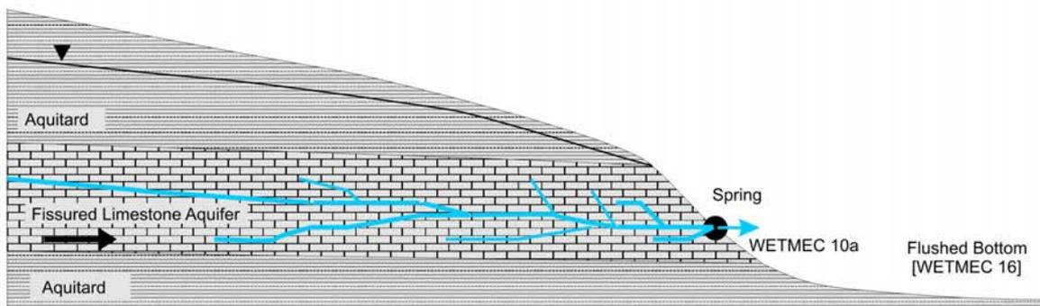
**Figure 6.31 (cont.) Schematic sections of types of Permanent Seepage Slopes
