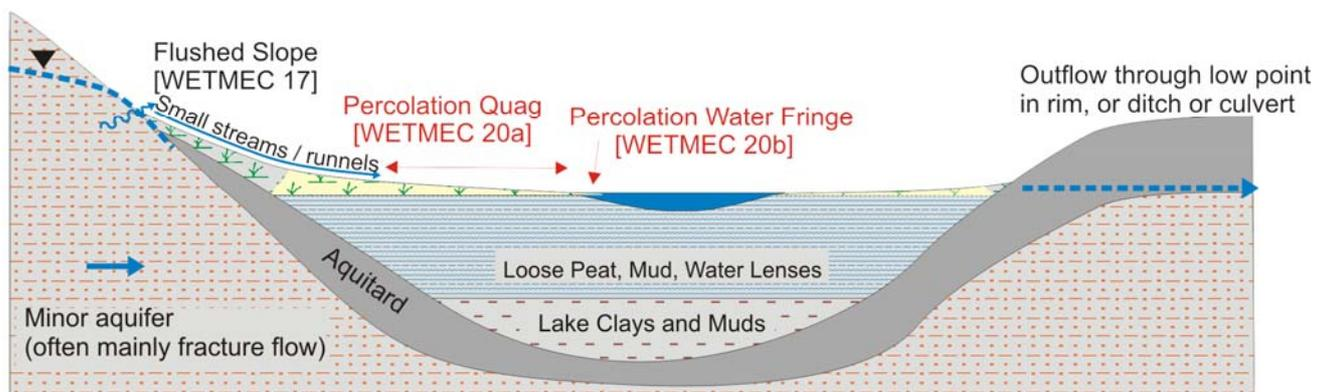
Figure 6.51 Schematic sections of Percolation Basins (WETMEC 20)
