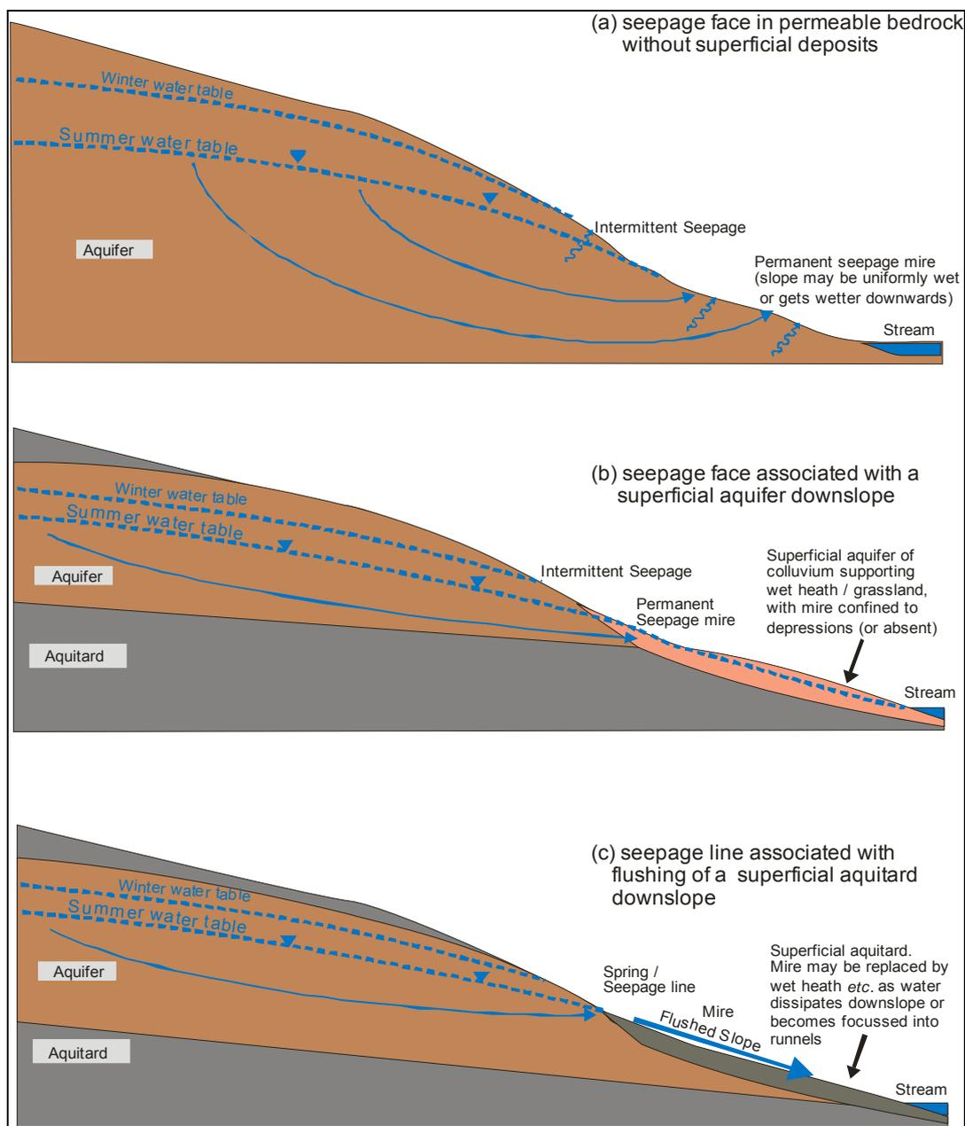
**Figure 5.1 Schematic sections showing the influence of superficial deposits of varying composition downslope of groundwater outflows upon the gross patterns of water flow and the habitats that develop**
