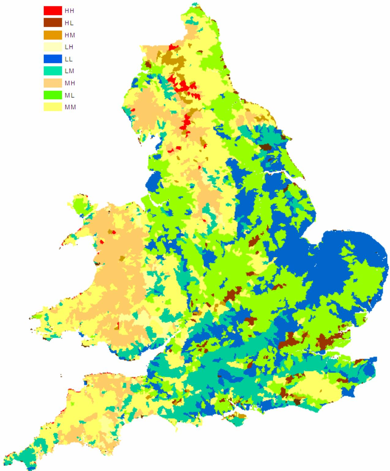
**Figure 4.5 Combined slope/SAAR and drainage density defined erosivity classes – letters in key represent transportability scores (e.g. HH = 6, MM = 4, LL = 2)**
