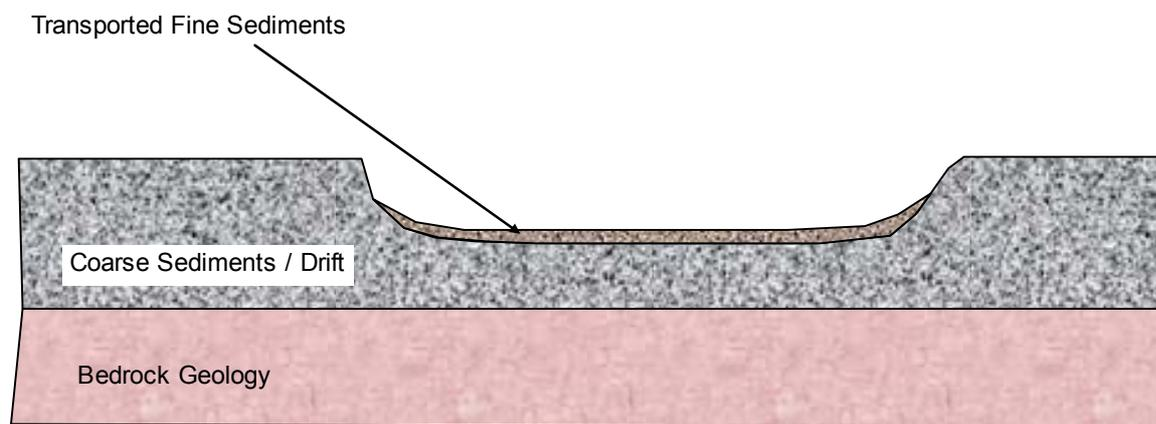
**Figure 1.3 Simple conceptual model used during the creation of the HZ classification scheme**
