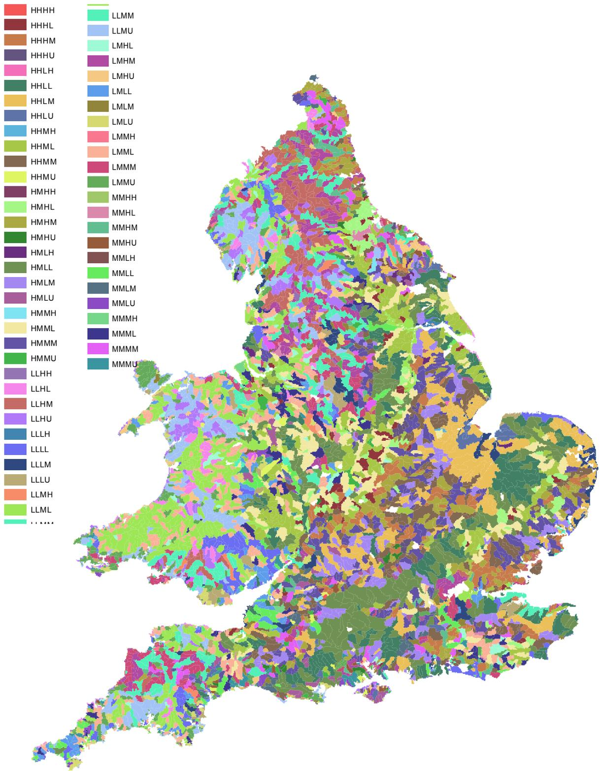
**Figure 6.2 The 58 final HZC classes. In order, the classes represent sediment thickness, sediment permeability, subsurface permeability and geochemistry**
