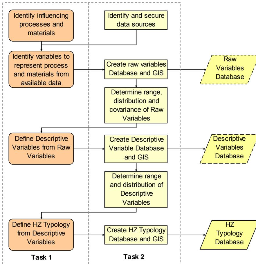
It can be seen that the development of the HZ typology is an iterative process between theoretical development and data interrogation (as opposed to the originally envisaged method of predefining a typology and then fitting over the available data). This approach is designed to create typology classes that give a better representation and definition to the more frequently occurring HZ types (e.g. lowland, permeable-bed water bodies).
