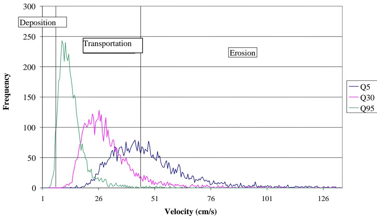
**Figure 4.9 Hjulstrom sediment transport and deposition thresholds for sand-sized sediment**
