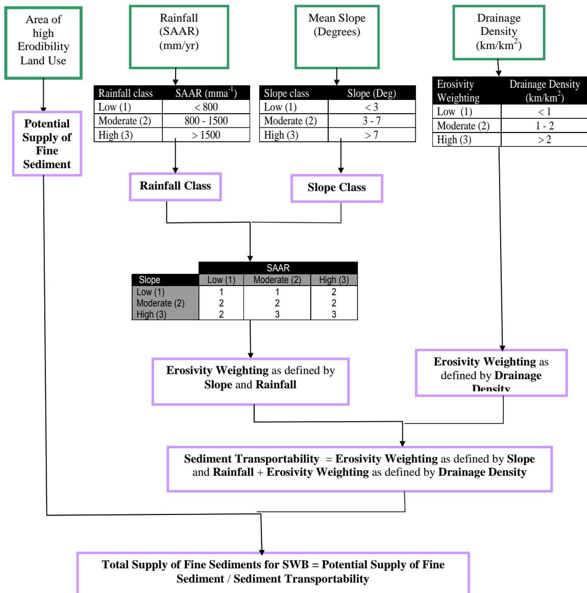
Figure 1 Flow chart showing the process for determining the Fine Sediment Supply Axis
