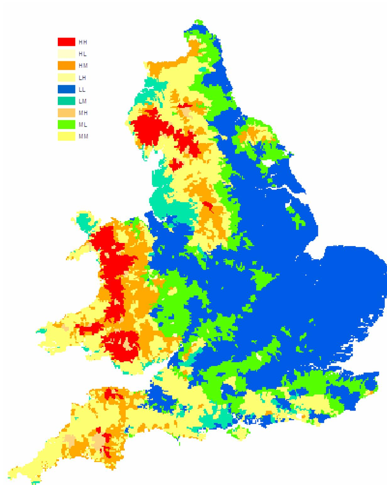
**Figure 4.4 Erosivity classes for SWB catchments in England and Wales – letters in key represent parent slope and SAAR classes (low, medium, high)**
