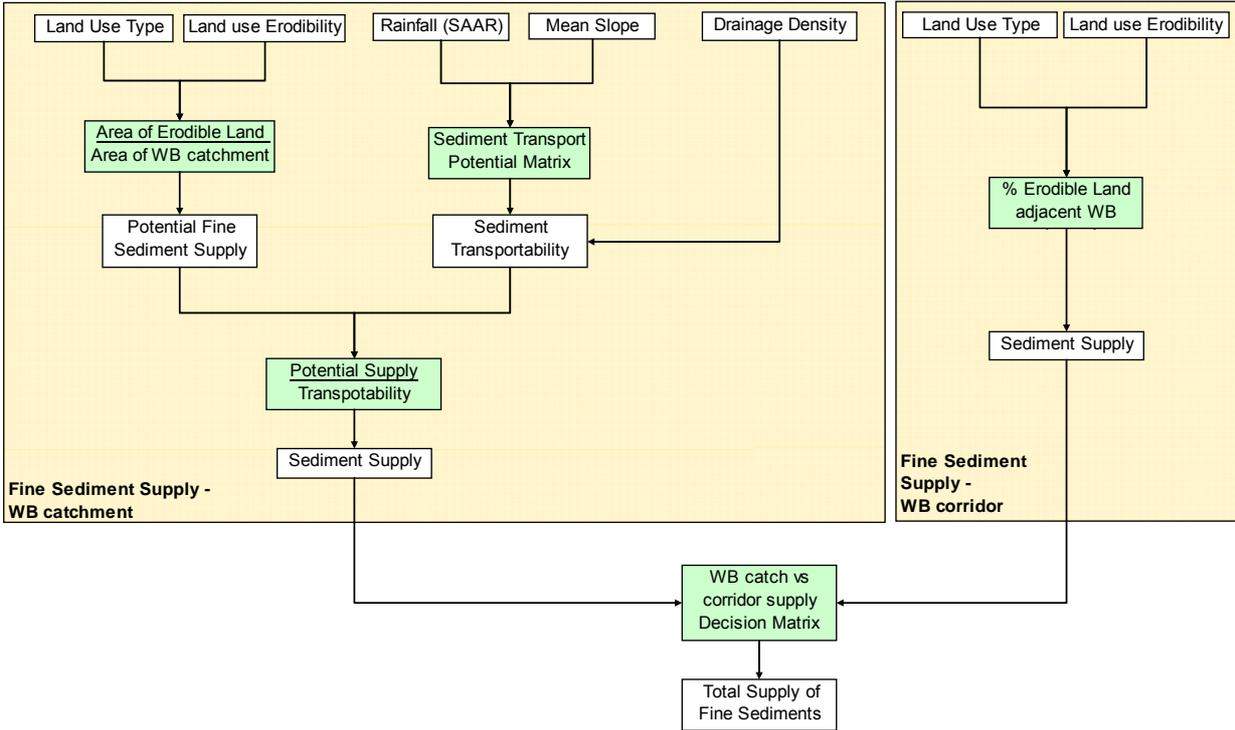
**Figure 4.2 Initial conceptual model for production of water body fine sediment**
