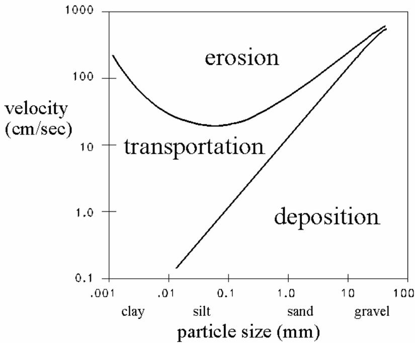
**Figure 4.8 Hjulstrom diagram illustrating thresholds of sediment erosion, transportation and deposition for differently sized particles**
