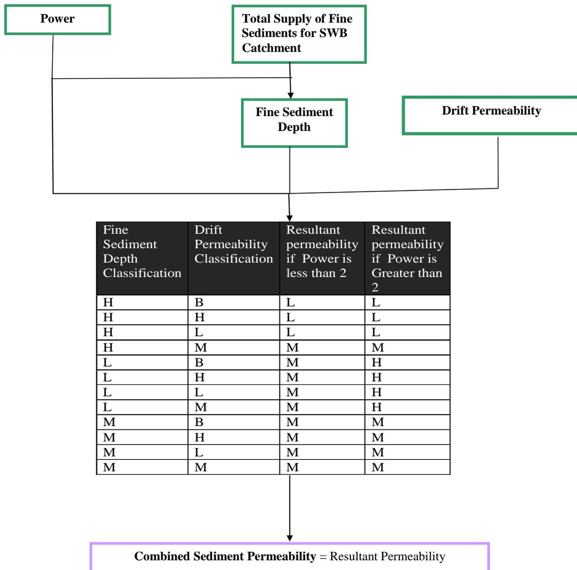
**Figure 3** Flow chart showing the process for determining the Combined Sediment Permeability
