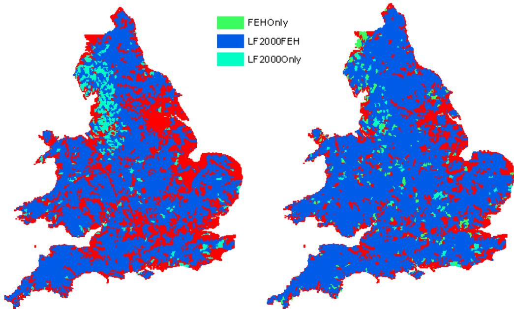
**Figure 3 Comparison of FEH and LF2000 data coverage before and after introduction of new X–Y points (red areas indicate no data)**
