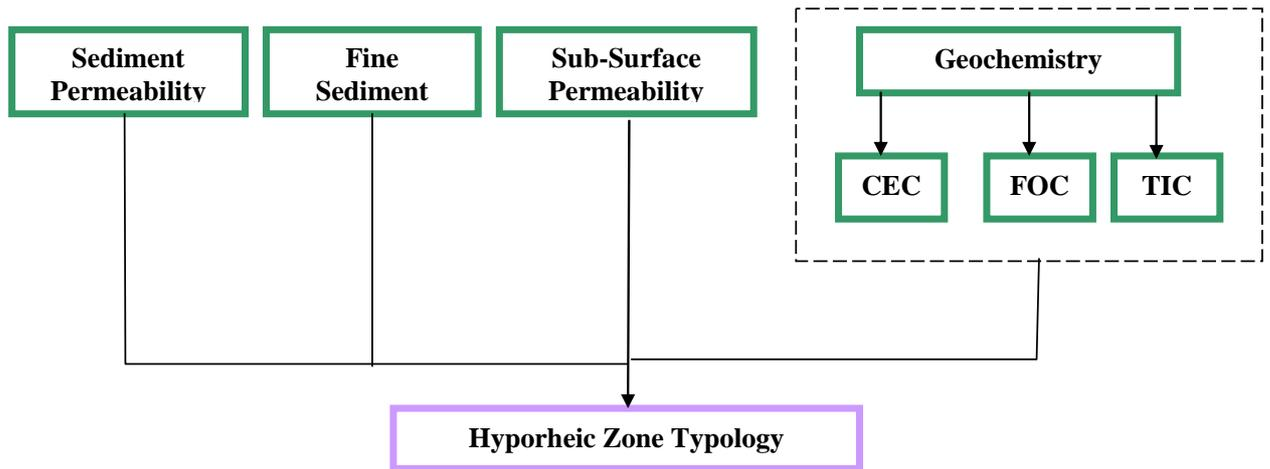
Figure 4 Flow chart showing the process for determining the HZ classification
