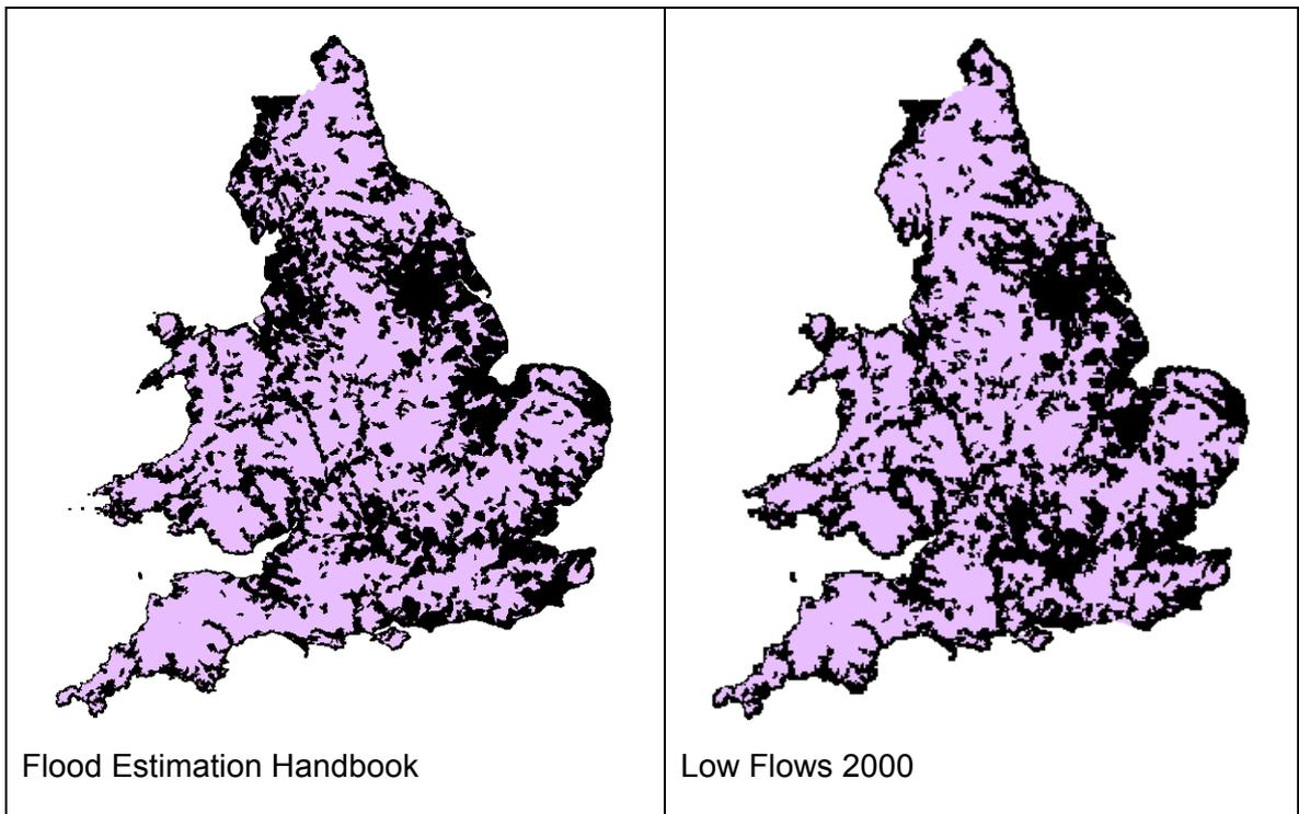
**Figure 2** Spatial coverage of LF2000 and FEH datasets using original method – dark areas indicate missing data
