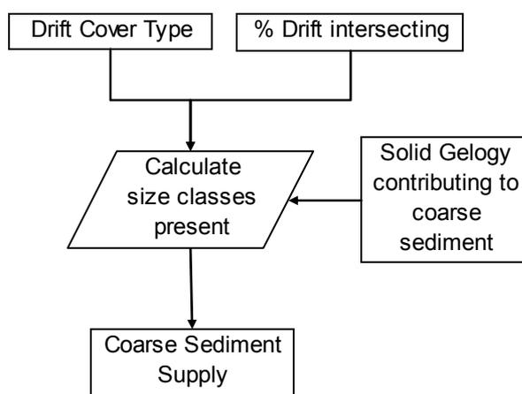
**Figure 4.7 Schematic representation of coarse sediment supply calculation**
