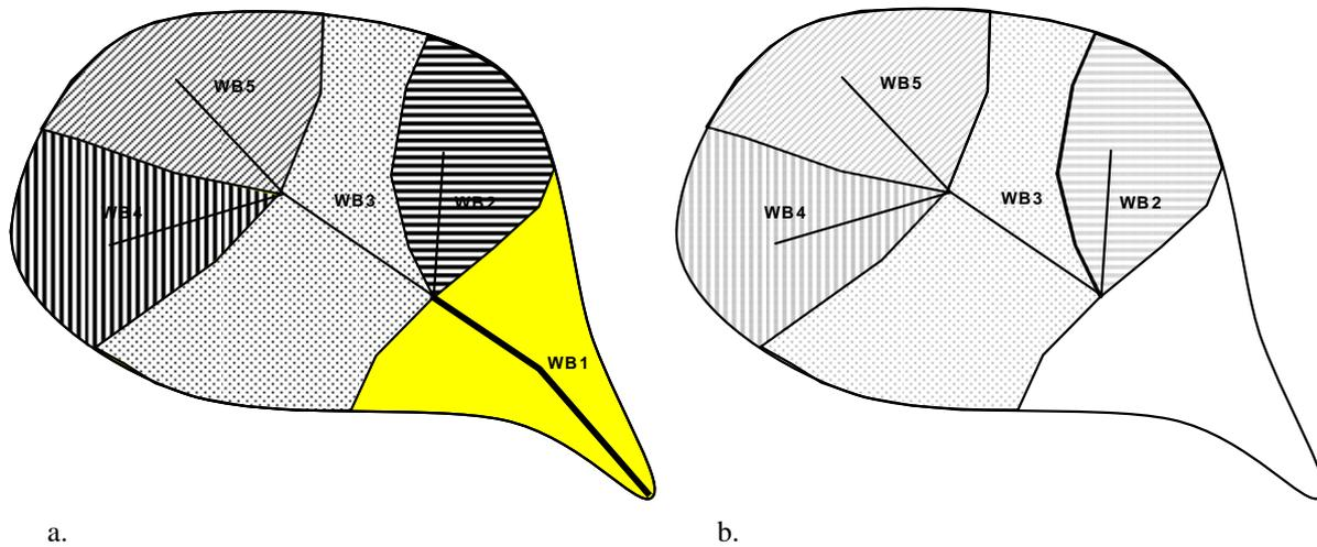
**Figure 4.1 (a) Illustration of water body catchment river channel (WB1) and water body catchment area (yellow), (b) contributing upstream area of WB1 (WB2; WB3; WB4; WB5)**
