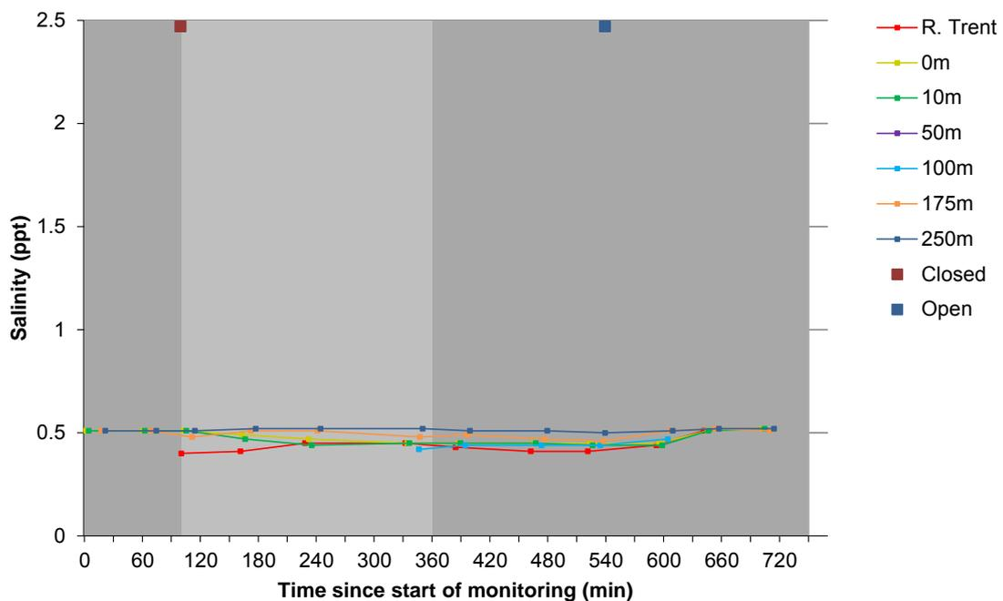
**Figure 5.20 Salinity measured in the River Eau during the neap-closed survey**
