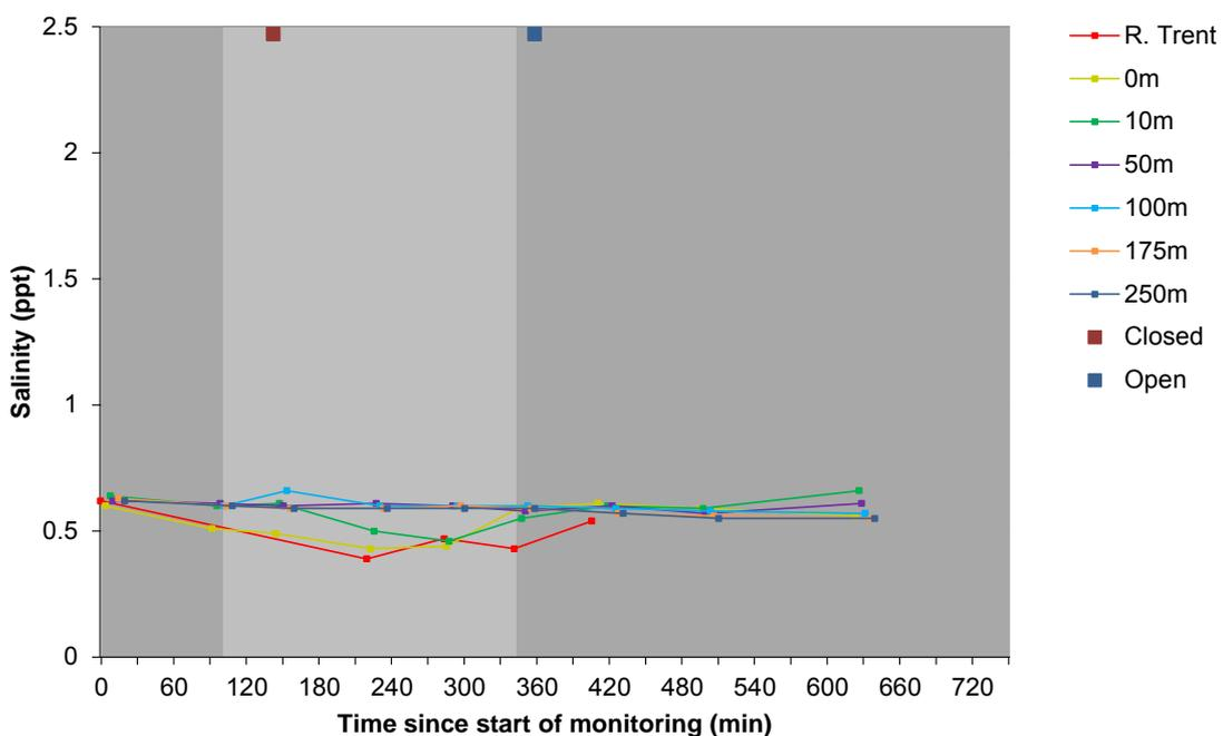
**Figure 5.12 Salinity measured in Burton-on-Stather Drain during the neap-closed survey**
