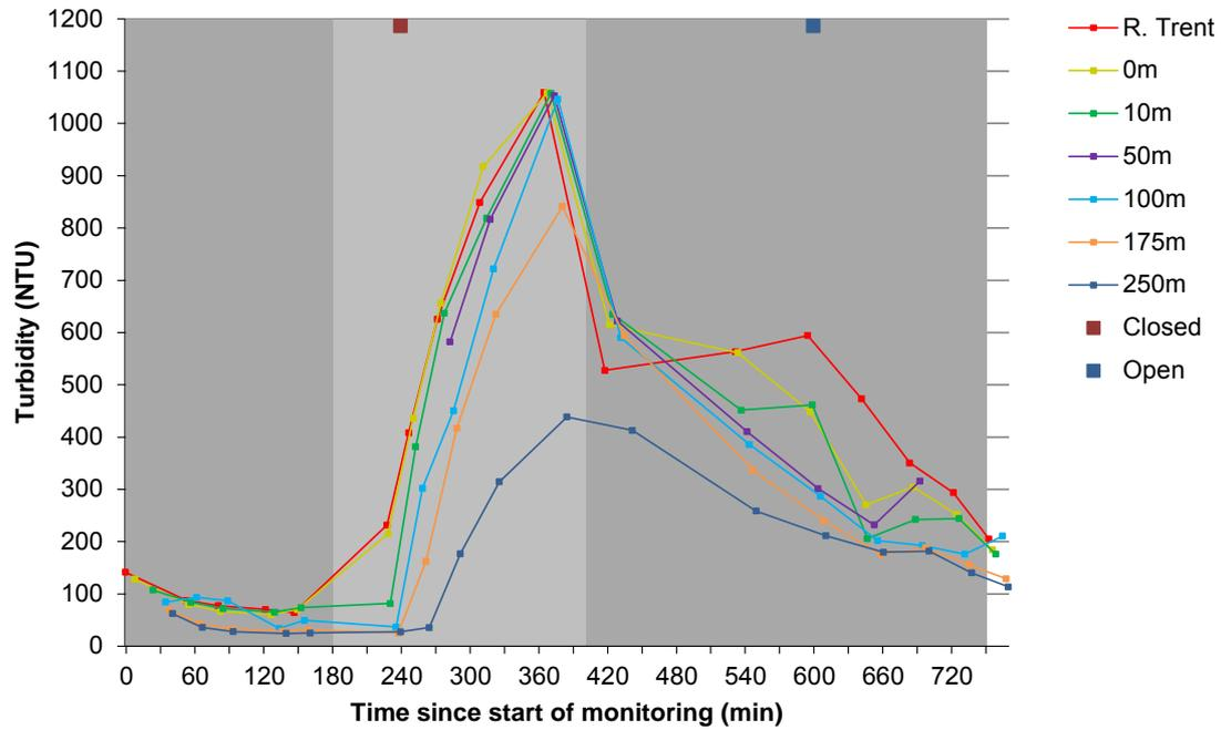
**Figure 5.22** Turbidity measured in the River Eau during the neap-open survey
