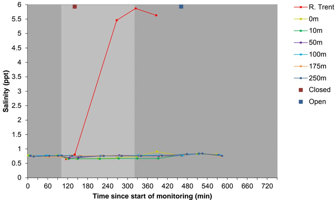
**Figure 5.10 Salinity measured in Burton-on-Stather Drain during the neap-open survey**
