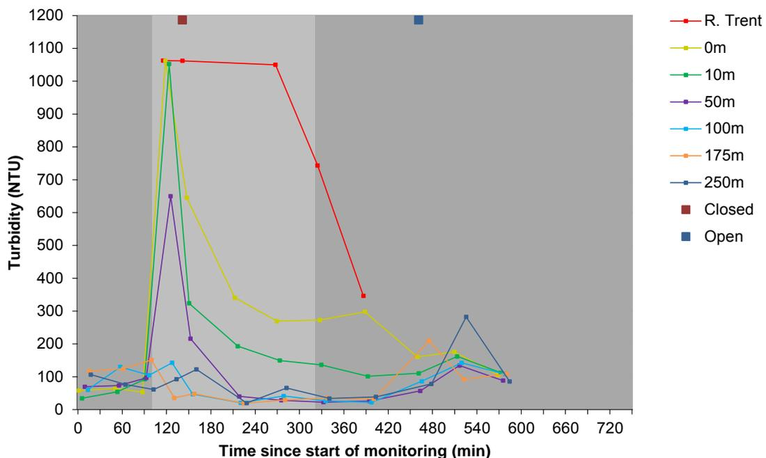
**Figure 5.14 Turbidity measured in Burton-on-Stather Drain during the neap-open survey**
