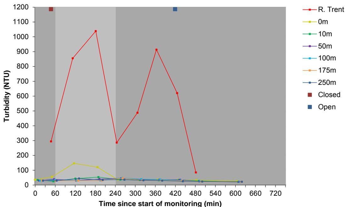
The bimodal response in turbidity within the River Trent during the survey (Figure 5.6) is due to the tidal cycle, with both peaks occurring during the highest flow velocities in the flood and ebb tidal periods when most sediment will be in transport. This response
