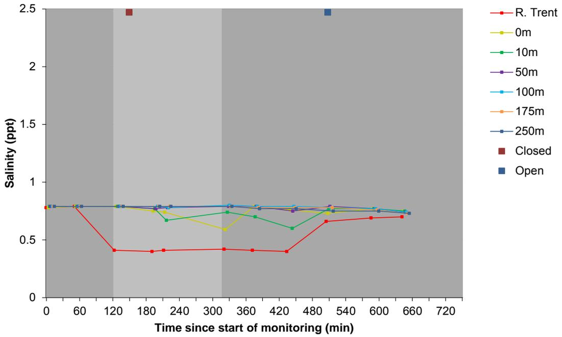
**Figure 5.4 Salinity measured in Burringham Reservoir Drain during the neap-closed survey**
