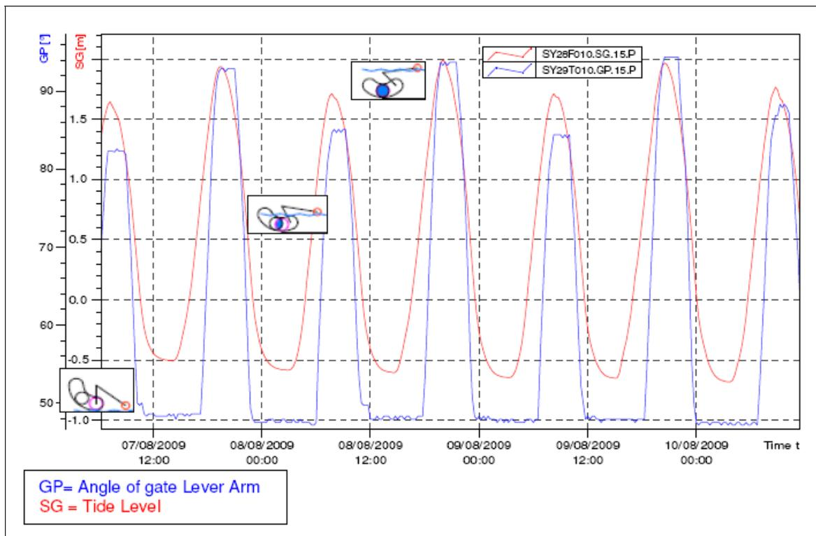
**Graph 1 Trace from the SRT monitoring device plotted against the tide level recorded at Seaton tide gauge (normal condition)**
