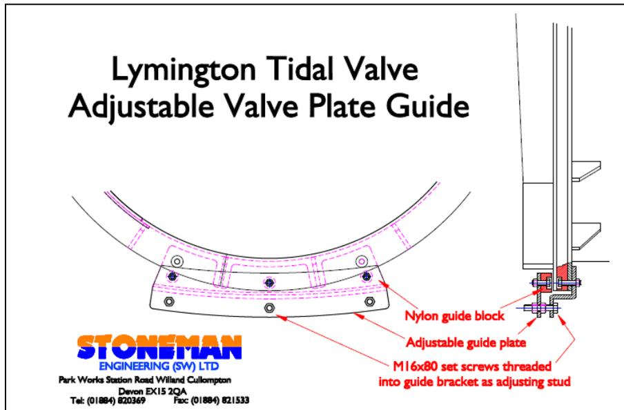
**Figure 3-4 Revised valve plate guide**
