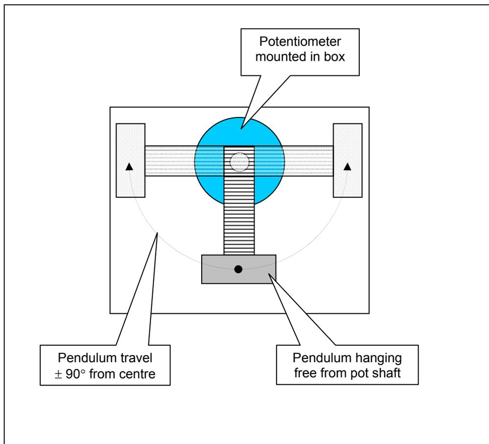
**Figure A1. Angle measuring potentiometer general mounting arrangement**
