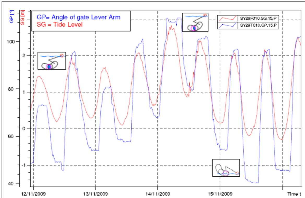
**Graph 2 Trace from the SRT monitoring device plotted against the tide level recorded at Seaton tide gauge (extreme tides)**
