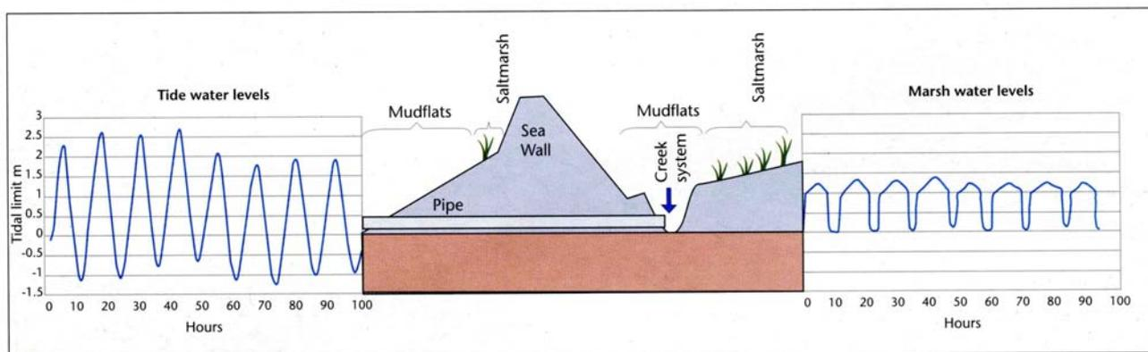
Figure 1 Schematic representation of Regulated Tidal Exchange showing the tidal variation and natural mudflat and saltmarsh 'squeezed' against hard sea defences. The figure shows Regulated Tidal Exchange allowing mudflats and saltmarsh to develop inside the sea wall and the modelled response of the marsh water levels. Diagram developed from actual tidal data and land elevations at a site in eastern England.
