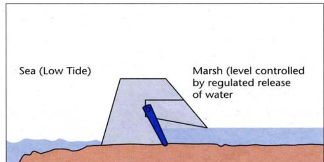
**Spillway System:** A lowered portion of the sea wall allows sea water to enter the marsh at high tides.
