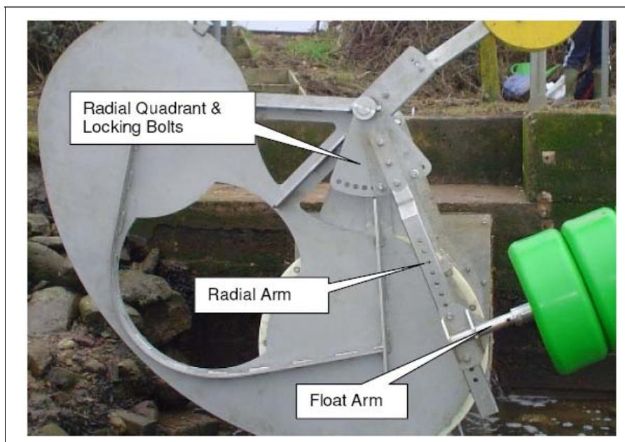
**Figure 2-3 Photograph of the Seaton gate methods of adjustment**
