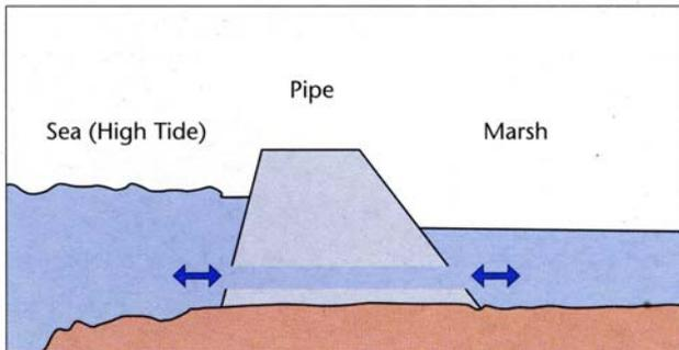
**Flapper system:** A flapper or tidal gate held by culvert blocks, usually uni-directional, with or without sluices for level control. A flapper or tide gate can be considered as a large-scale pipe system.
