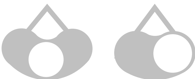
Figure 4: Stop-go-stop (left) and go-stop variants of self-regulating tidegates
