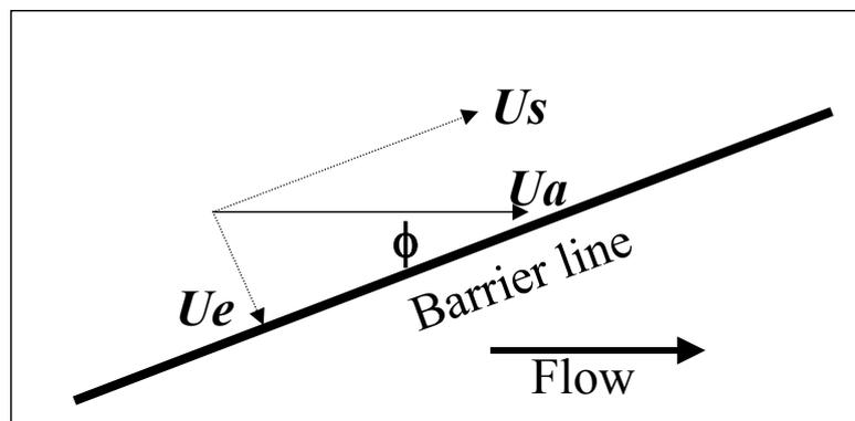
**Figure 5.5** Flow velocity components in front of an angled fish barrier.  $U_a$  is the channel velocity,  $U_e$  is the fish escape velocity and  $U_s$  is the sweeping velocity component along the face of the screen (after Turnpenny *et al.*, 1998).
