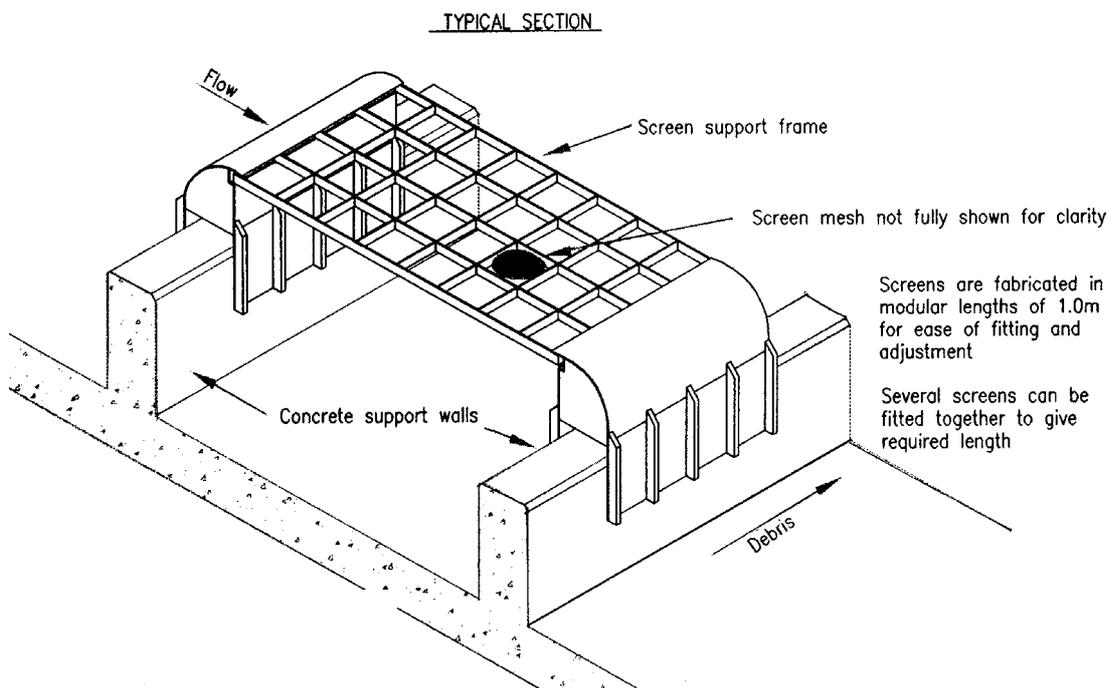
**Figure 3.4 The Smolt Safe™ Screen (Rivertec Ltd)**
