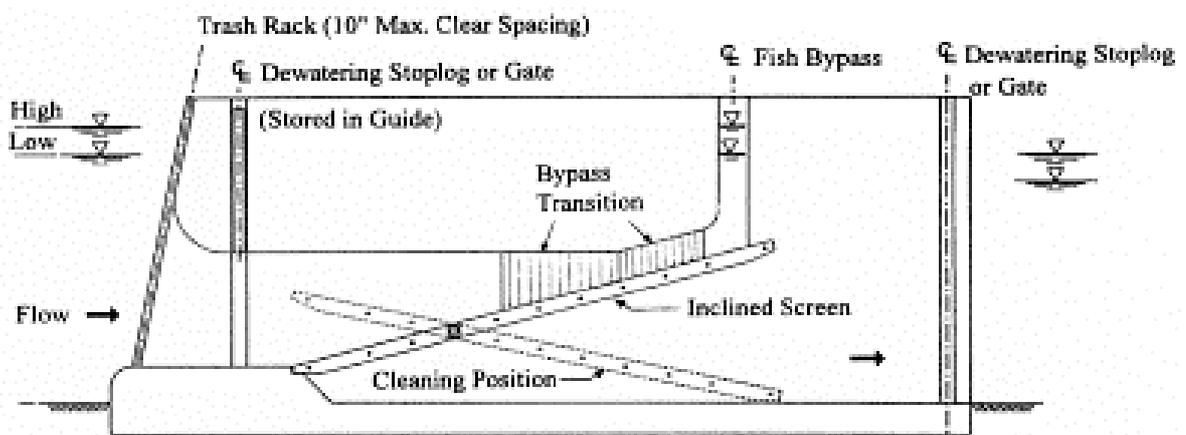
**Figure 3.10 Diagram of a Modular Inclined Screen ([www.aldenlab.com/scop-fisheries](http://www.aldenlab.com/scop-fisheries))<sup>14</sup>**
