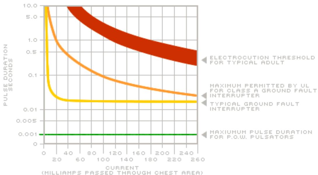
**Figure 3.14 Electrical pulse duration and current data for the GFFB™ pulse generator in relation to human risk criteria ([www.smith-root.com](http://www.smith-root.com)).**
