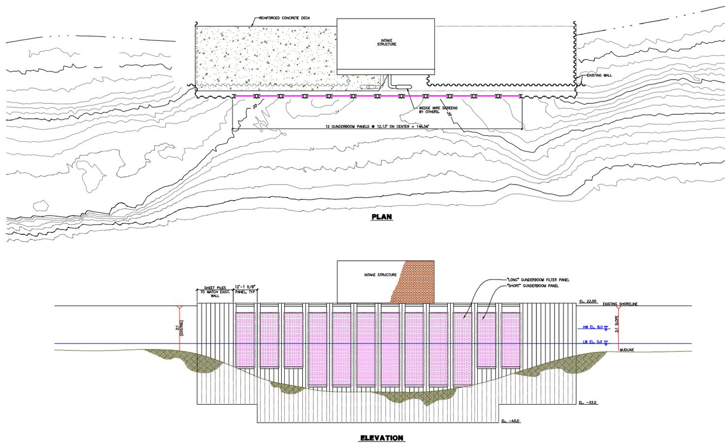
Figure 3.9 Example of a MLES layout (Gunderboom Inc.)
