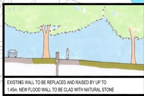
EXISTING WALL TO BE REPLACED AND RAISED BY UP TO 1.45m. NEW FLOOD WALL TO BE CLAD WITH NATURAL STONE
