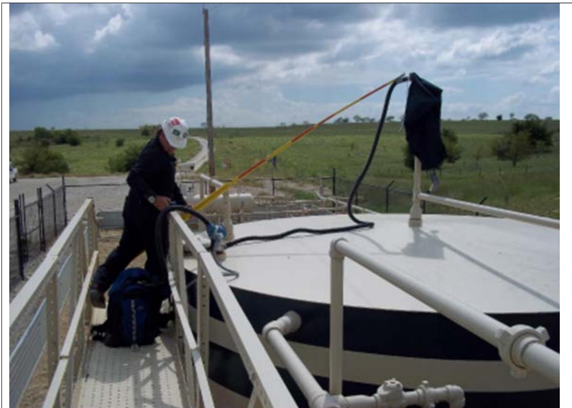
**Figure 5.7 Leak rate quantification using a Bacharach™ Hi Flow sampler**
