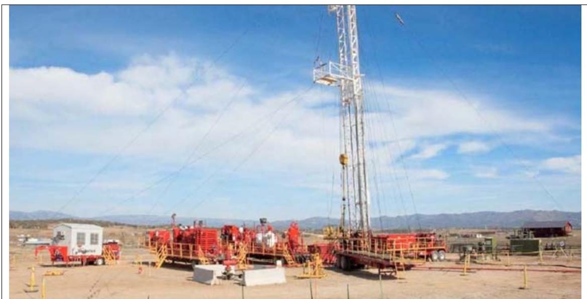
**Figure 5.1 Reduced emissions completion unit, Wyoming (BP 2011)**
