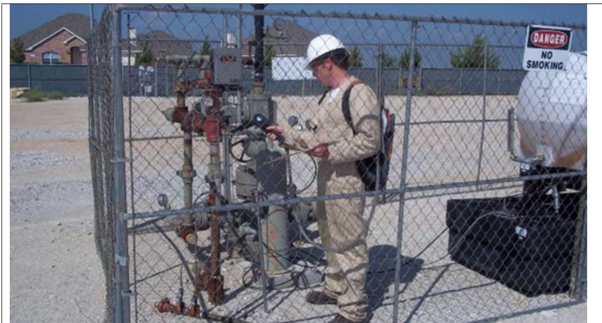
**Figure 5.6 Concentration data obtained through the use of a toxic vapour analyser**
