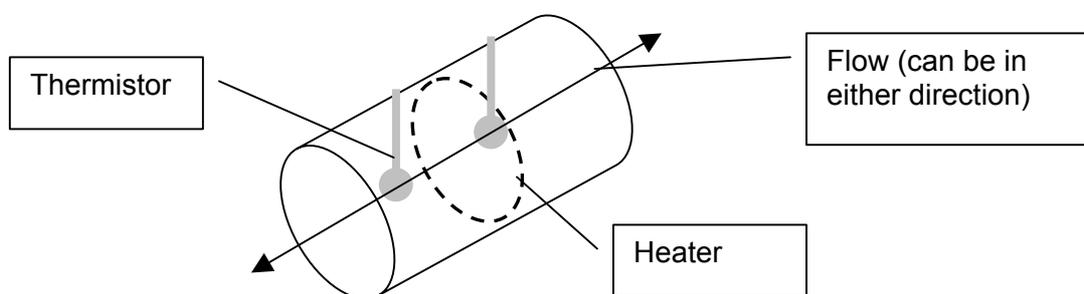
Figure 4.2 Schematic diagram of a heat pulse flow meter.
