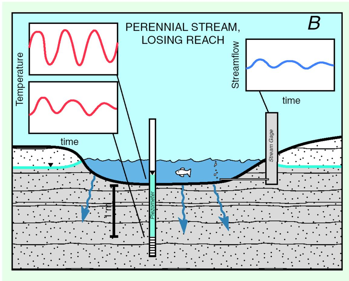
**Figure 6.2** Temperature profile in a losing reach (Constantz and Stonestrom 2003). Heat is transported by both advection and conduction from the surface water body into the sediments. Unlike gaining reaches, in which the system is damped by the influx of groundwater at a relatively constant temperature, losing reaches are characterised by larger diurnal fluctuations in temperature within the sediments and the water body itself.
