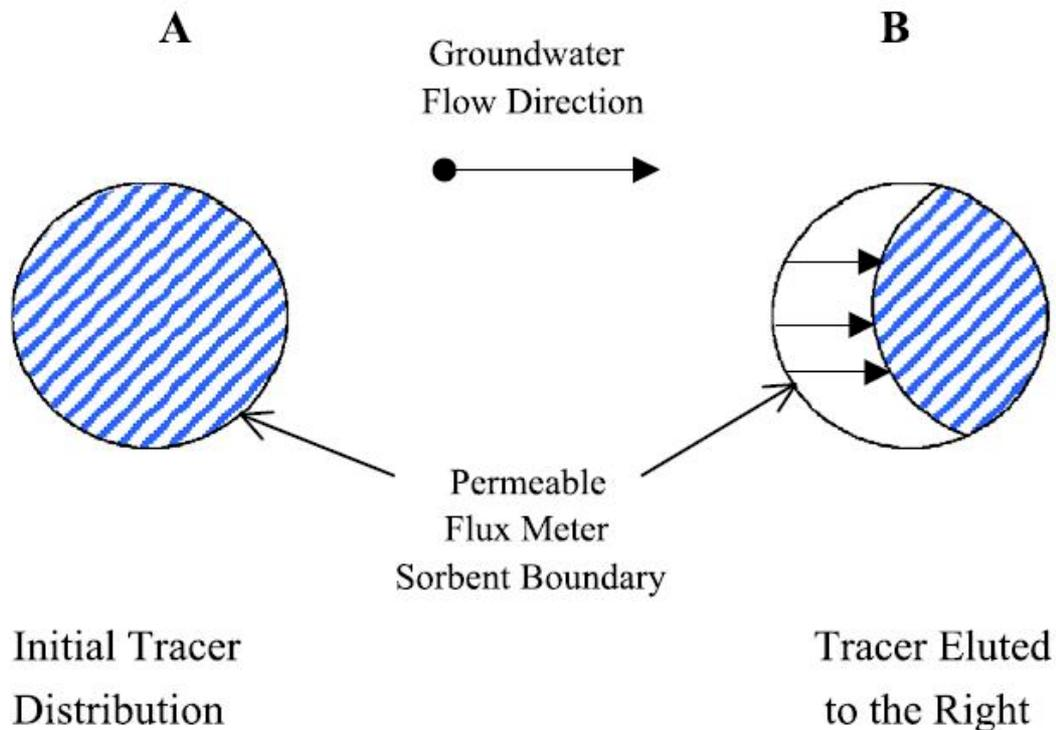
**Figure 2.4** Conceptual diagram of resident tracer distribution in two cross-sections of a passive flux meter showing (a) the meter before and (b) after exposure to groundwater flow (Hatfield *et al.* 2004).
