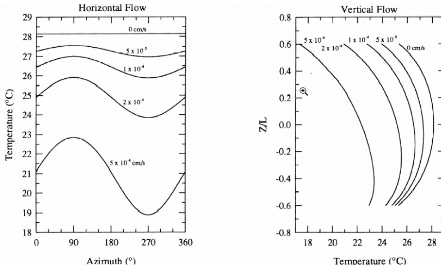
**Figure 3.1** The distribution of temperature on the surface of the *in-situ* permeable flow sensor as a function of azimuth and flow velocity under conditions of purely horizontal flow (left) and vertical downward flow (right), from Ballard (1996).
