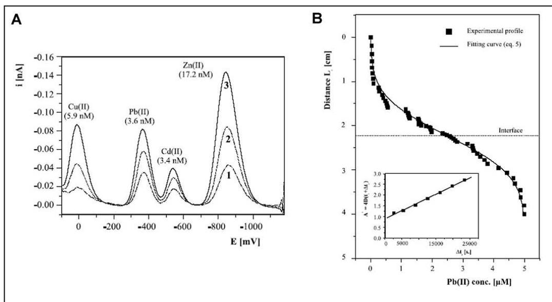
**Figure 2.7** (A) Simultaneous voltammetric measurements of Cu, Pb, Cd and Zn in prepared samples using an ultramicroelectrode array (UME). Compare the scales with those in *Figure 2.5(C)*. (B) Measurements of a small-scale concentration gradient in Pb(II) at  $<5 \mu\text{mol}$ . Figures taken from Tercier-Waeber *et al.* (1999) Copyright 1999 IOP Publishing Ltd.
