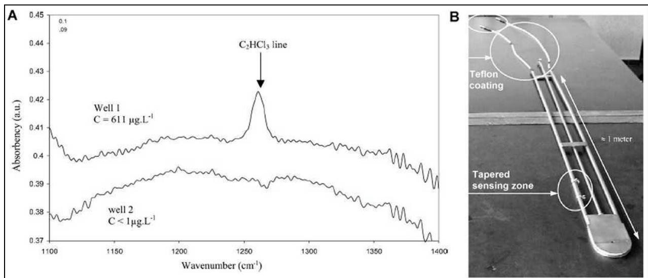
**Figure 2.14** Fibre evanescent wave spectroscopy (FEWS) probe employing chalcogenide-glass optical fibre to transmit IR excitation radiation to detect organochloride pollutants in groundwater. (A)  $C_2HCl_3$  can be clearly detected at a concentration of  $611 \mu\text{g/l}$ , but it is not detectable when present in trace quantities. (B) The probe is simple and light in construction and relatively rugged. Figures taken from Michel *et al.* (2004) Copyright 2004 Elsevier B.V.
