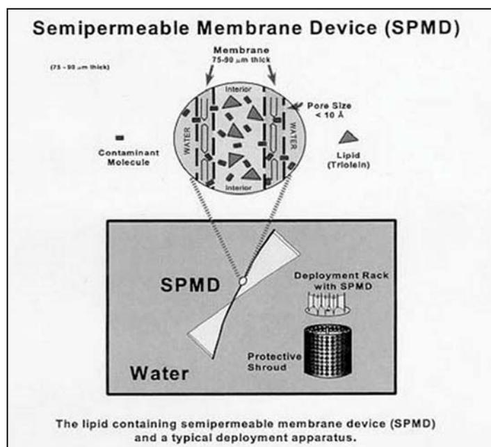
**Figure 2.11** A semi-permeable membrane device consists of a flat plastic tube with lipid sealed inside. This membrane allows bioavailable contaminants to pass through and concentrate in the lipid. Figure taken from website <http://wwwaux.cerc.cr.usgs.gov/spmd/>, accessed 15th March 2005.
