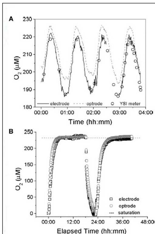
**Figure 2.12** Comparison of O<sub>2</sub> measurements by micro-optode and ion-selective electrode. (A) Higher frequency changes in oxygen concentration result in a poor fit of the optode data. (B) In less dynamic environments, the performance of the optode closely matches that of the electrode. Figures taken from Glazer *et al.* (2004) Copyright 2004 Elsevier B.V.
