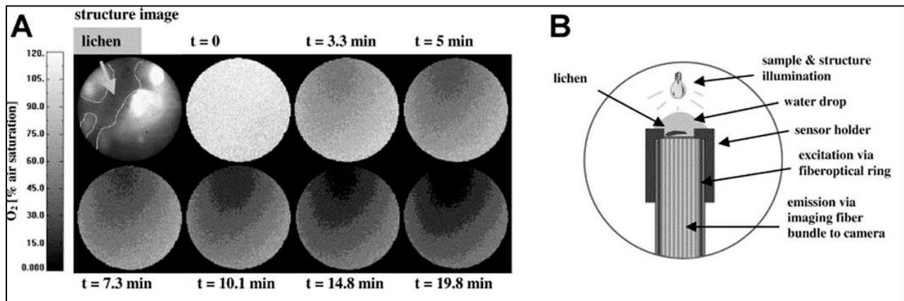
**Figure 2.13** (A) A transparent planar optode deployed with a fibreoptic endoscope to measure respiration by means of  $O_2$  luminescence lifetime. The fibreoptic bundle carries both excitation and emission light for the optode. (B) An external light source allows the structures related to the oxygen signal to be imaged through the transparent optode. Figures taken from Holst and Grunwald (2001) Copyright 2001 Elsevier Science B.V.
