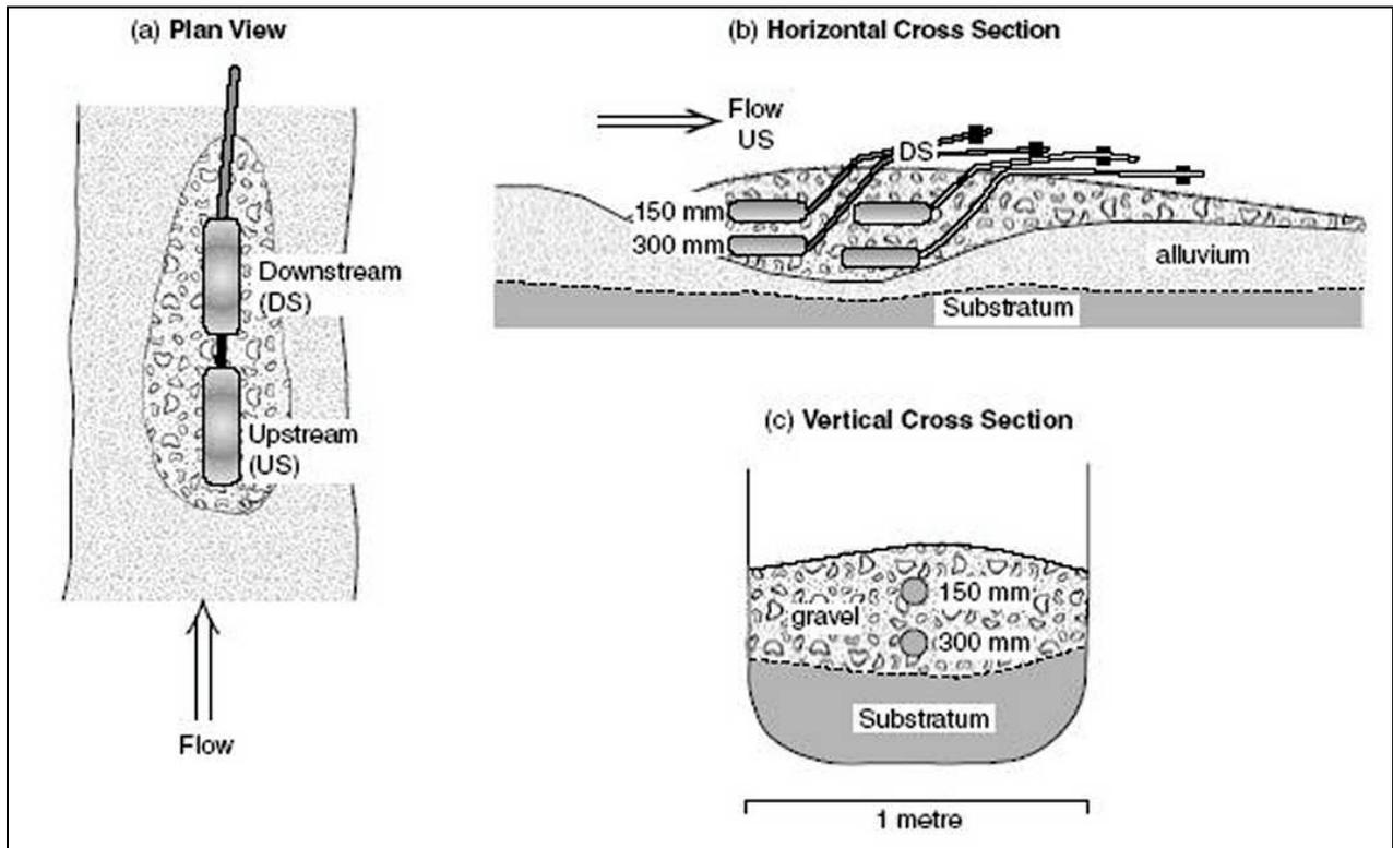
**Figure 2.1** Hyporheic sampling infrastructure described by Malcolm *et al.* (2003). Water sampling chambers are buried in artificial riffles which become integrated into the hyporheic zone system. Similar methodology could be used for deployment of *in situ* probes. Copyright 2002 John Wiley and Sons, Ltd.
