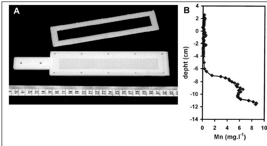
**Figure 2.8** Diffusive equilibration in thin films (DET). (A) Standard apparatus is a gel strip attached to a plastic paddle-shaped backing plate and held in place by a retaining plate. The strip can be obtained pre-sectioned, as in this image. (B) Typical vertical profile for Mn within shallow estuarine sediments. High spatial resolution can be obtained. Taken from Docekalova *et al.* (2002) Copyright 2002 Elsevier Science B.V.
