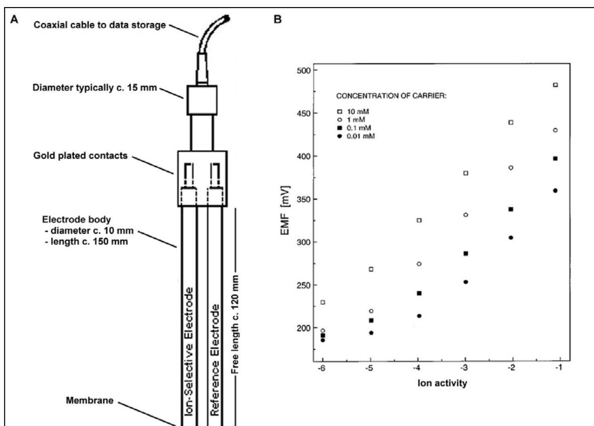
**Figure 2.4** Main components (A) and typical response curves (B) for an ion-selective electrode. Note the measured electromagnetic field (EMF) from an analyte at any concentration is dependent upon ion activity (i.e., presence as free ions available to interact with the probe). Diagram adapted from an original in Rundle (2000).
