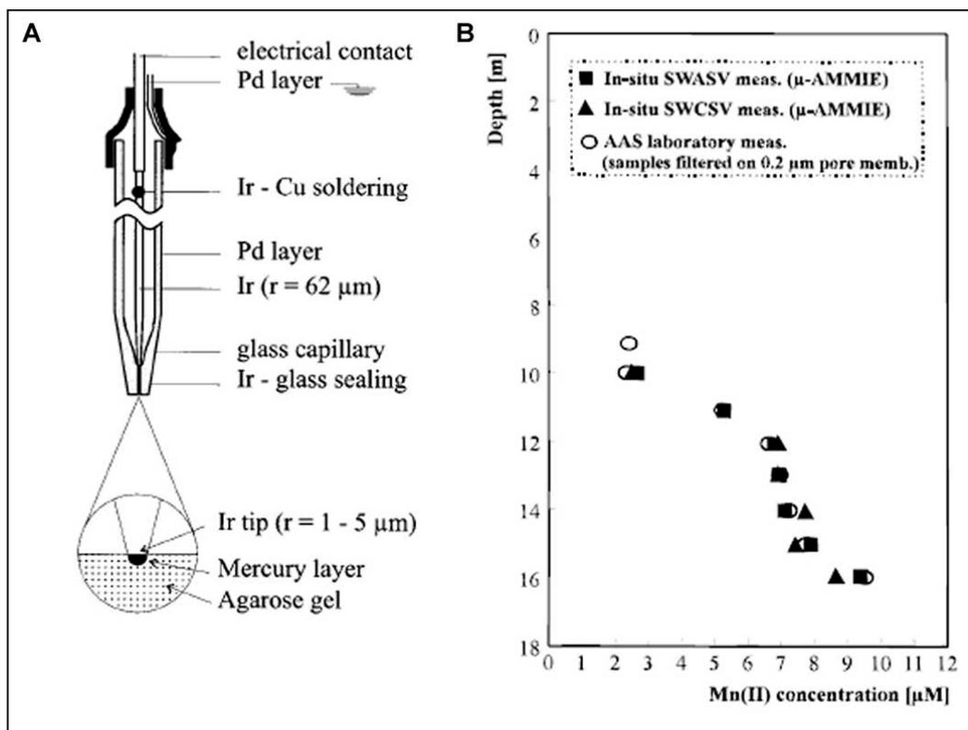
**Figure 2.6** (A) Schematic showing components of a gel-integrated iridium electrode used for *in situ* measurements of Mn in lake sediments. (B) Depth profile in lake sediments of Mn, measured using a gel-integrated electrode with square-wave anodic and cathodic stripping voltammetry, compared with *ex situ* atomic absorption spectrometry analysis (AAS) of samples. Figures taken from Tercier-Waeber *et al.* (1998) Copyright 1998 American Chemical Society.
