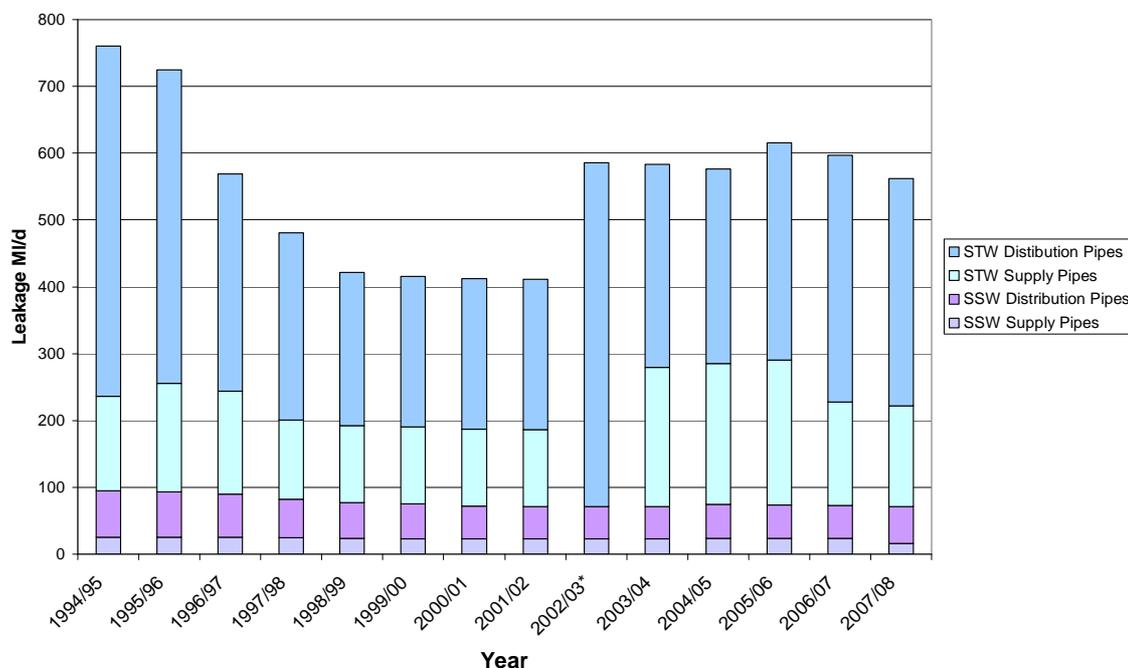
**Figure 15: Water supply leakage by pipe type for Severn Trent Water (STW) and South Staffordshire Water (SSW). \*The 2002/03 split data not available for Severn Trent Water therefore leakage assigned to distribution losses.**
