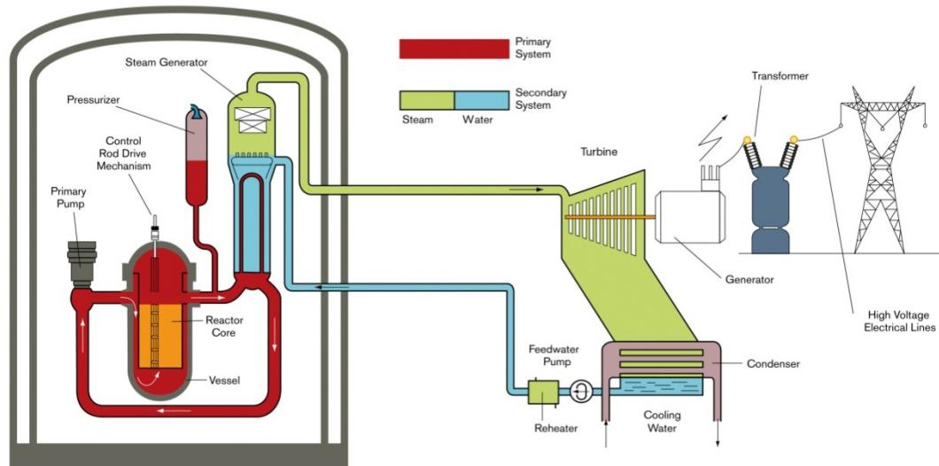
Figure 1 Simplified schematic of the EPR™ reactor (source AREVA)
