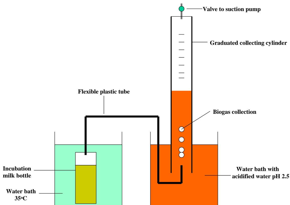
**Figure A.1 Schematic of BM100 method set up.**
