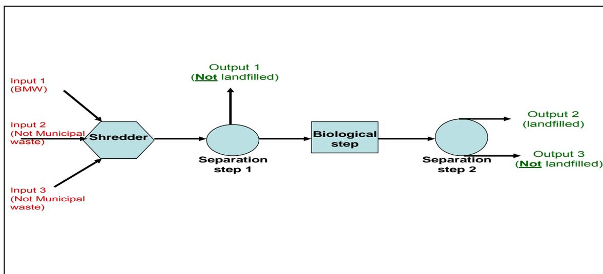
Figure 8.2 Example MBT with three inputs of which only one is municipal waste.
