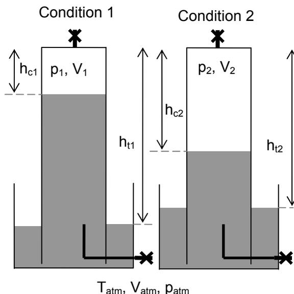
**Figure A.2 Biogas collection system monitoring**
