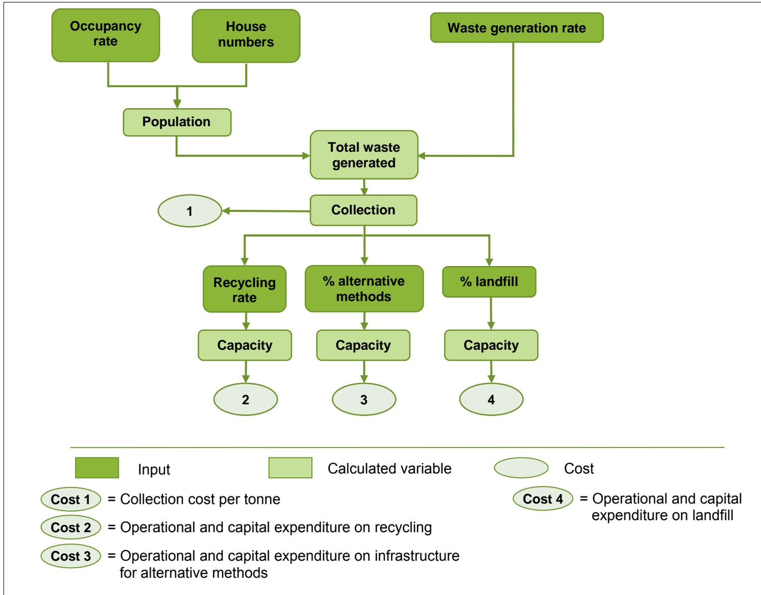
**Figure 7.2 Waste overview: Internal Capacity Approach**
