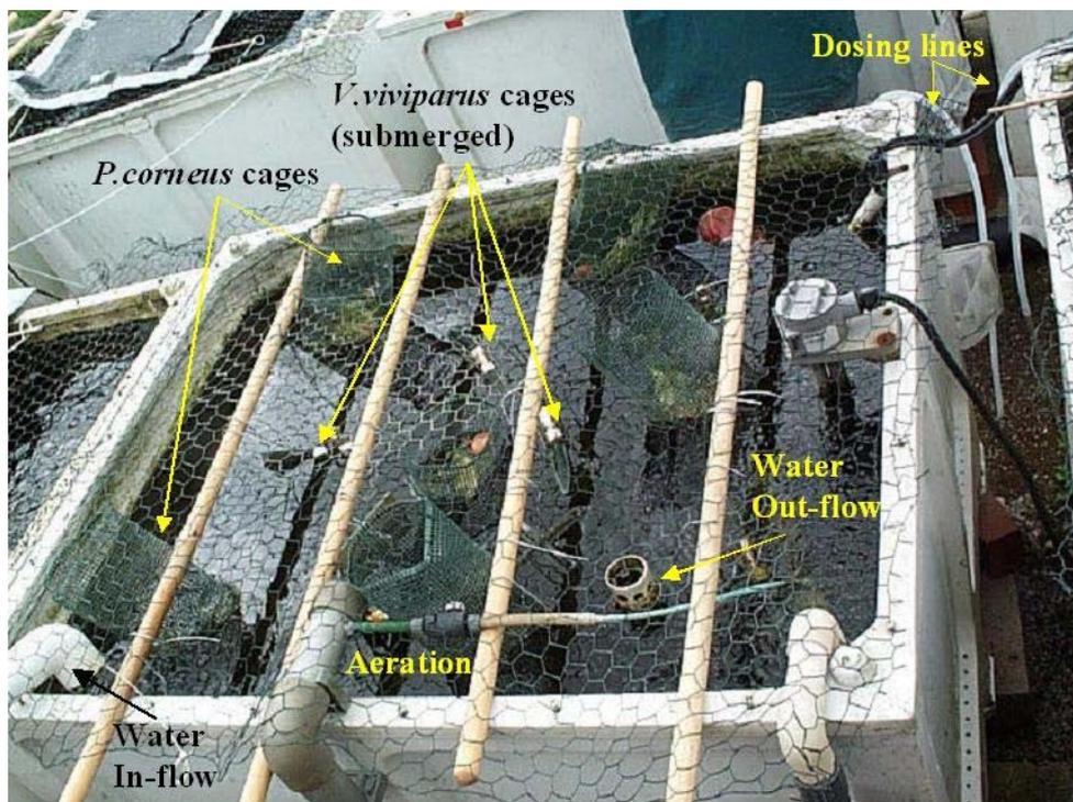
**Figure 2. Photograph of a mesocosm tank. Cages for adult snails are suspended by wooden broom handles. *P. corneus* cages are positioned so that the (air breathing) snails can reach the surface, but not escape. *V. viviparus* cages are submerged, providing the best habitat possible for this deeper water (gilled) species. River water flows into the tank through the pipe at bottom left and out through the pipe at bottom middle. The chicken wire cover prevented predation by birds.**
