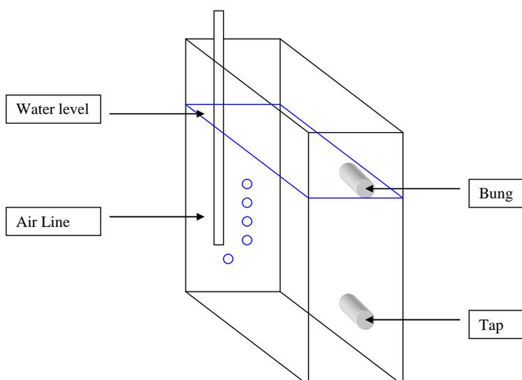
**Figure 69. Diagram of an exposure tank (15cm width x 30cm height x 30cm depth; water depth 24cm). The tanks were constructed using silicon sealant and had an outlet tap approximately 8cm from the bottom, which was made from ABS and polythene plastics.**
