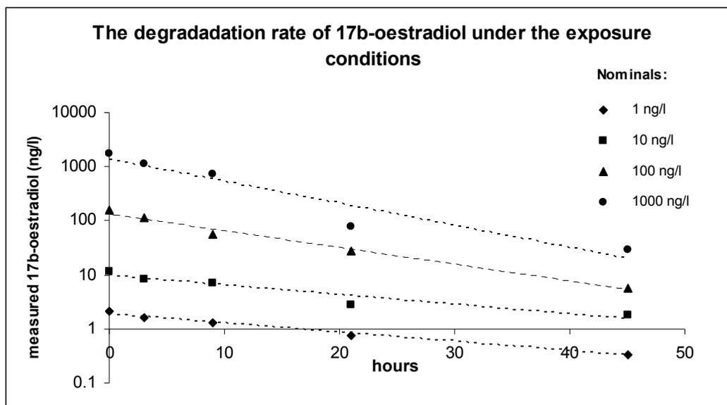
Figure 71. The measured degradation rate of E2 at 20°C under the conditions used in the exposure test.
