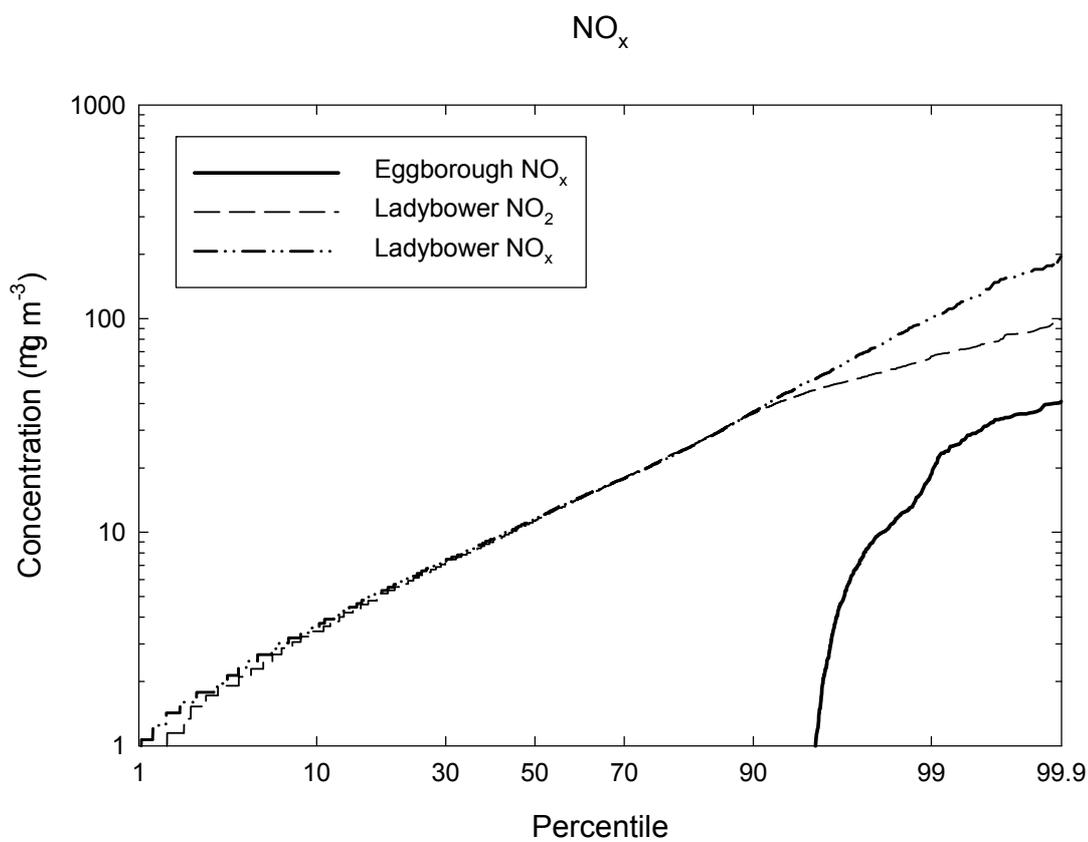
Figure 2. Concentrations frequency distributions from 'background' concentrations (Ladybower) and from a tall (200 m) power station discharge at the point of maximum concentration.
