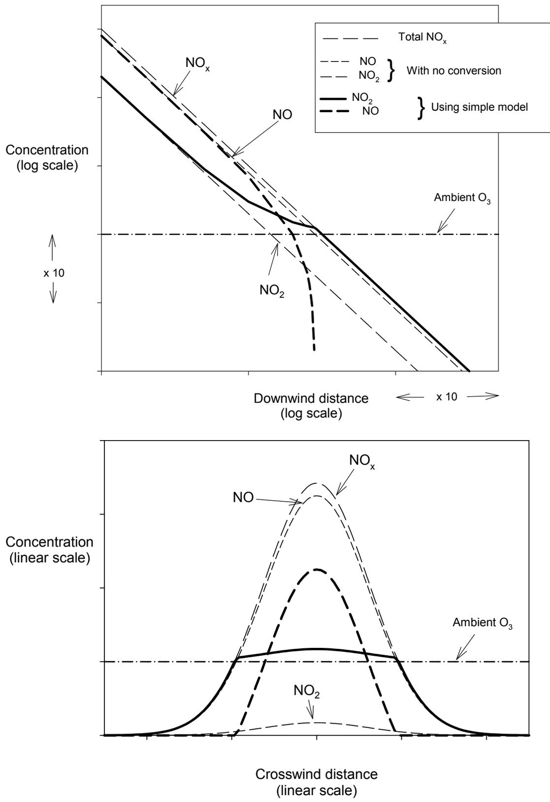
Figure 15. Diagram of the simple model for NO to NO<sub>2</sub> conversion in a plume. After Varey *et al.* (1984). Upper plot: along wind. Lower plot: across wind.
