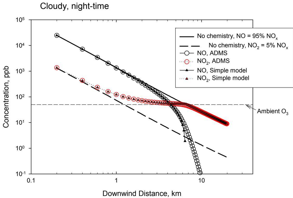
Figure 16. Comparison of ADMS3 chemistry module with simple oxidation model. Low solar radiation.
