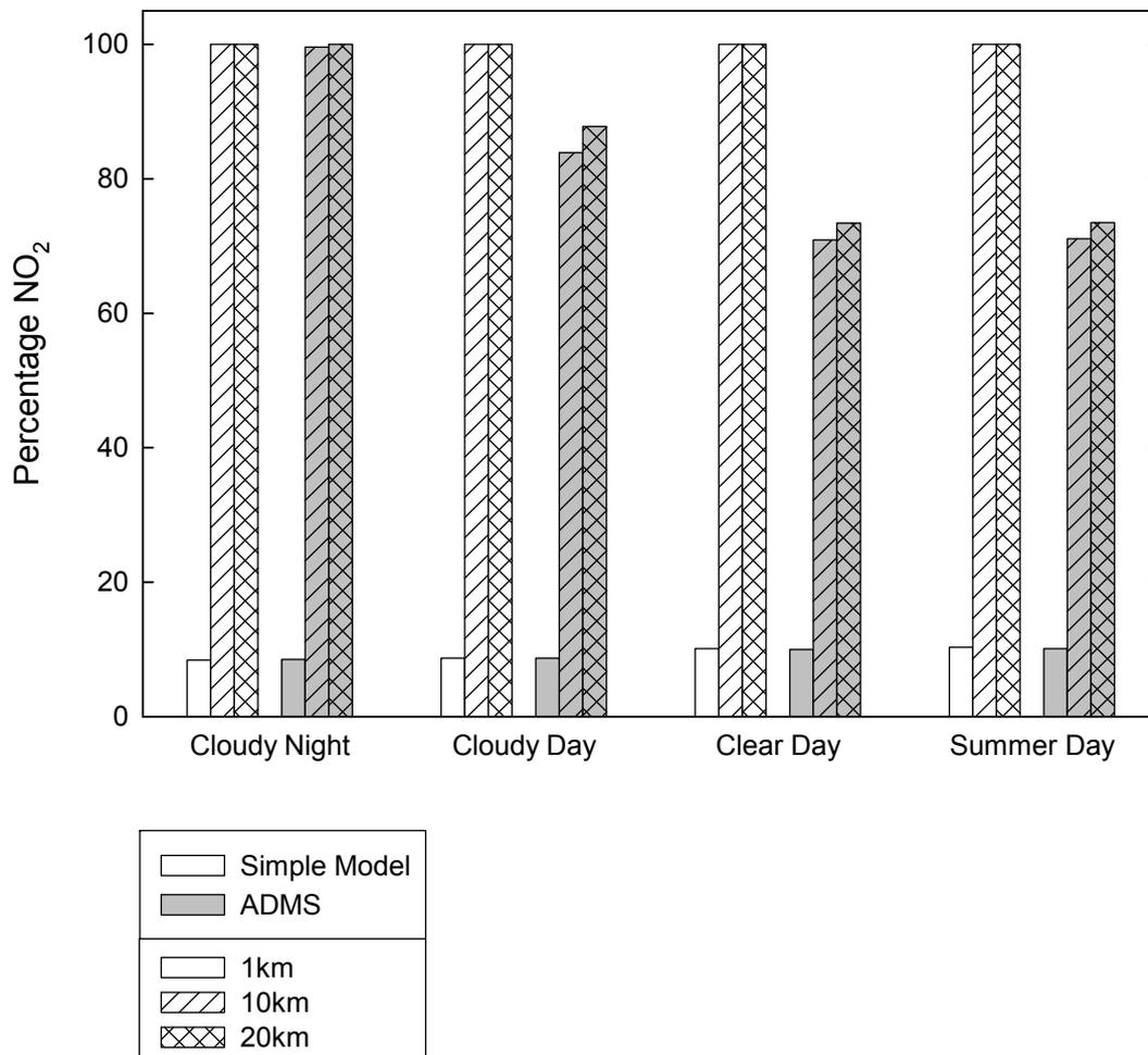
Figure 18. Variation in percentage NO<sub>2</sub> calculated by the simple model and ADMS3, for 10 m s<sup>-1</sup> wind speed and 50 ppb background ozone concentration.
