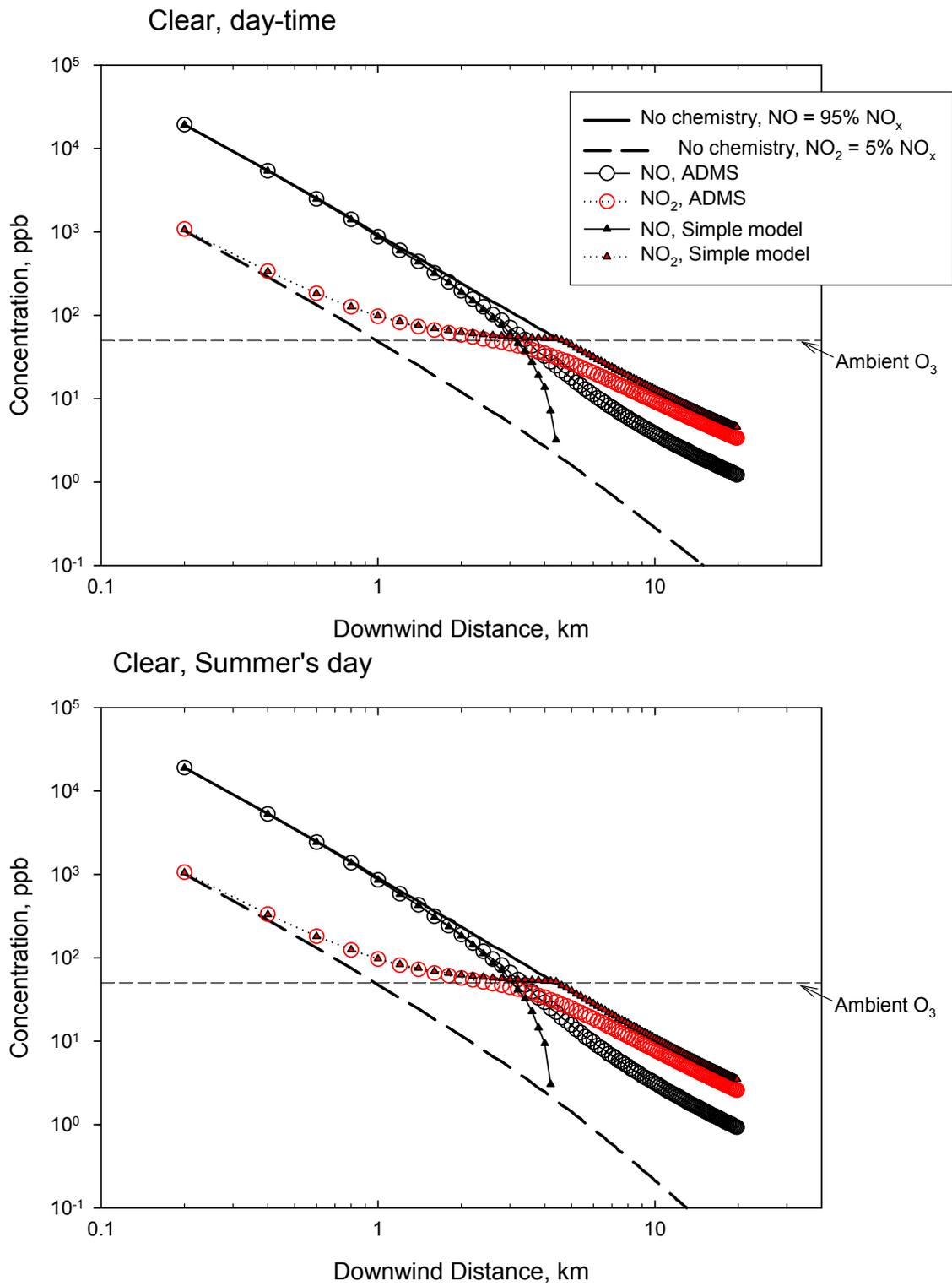
Figure 17. Comparison of ADMS3 chemistry module with simple oxidation model. High solar radiation.
