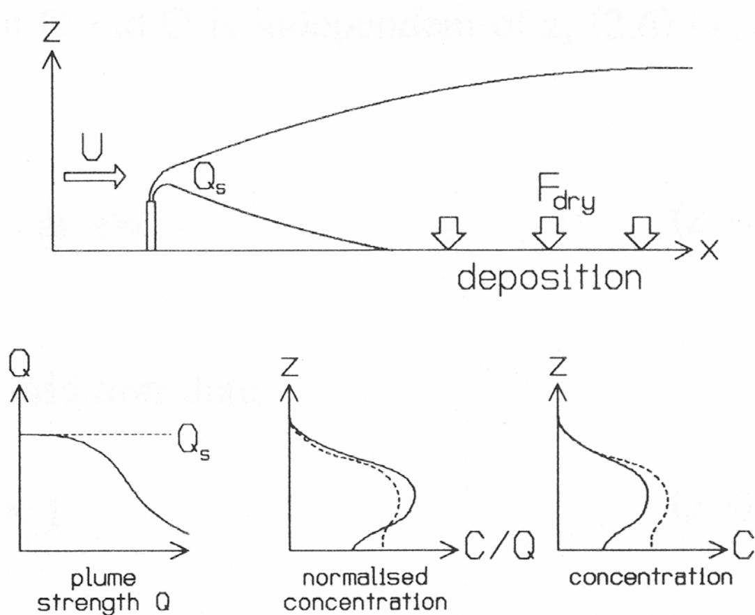
**Figure 1. Corrections for plume depletion due to deposition losses in ADMS model. From ADMS specification for deposition and radioactive decay (CERC, 1999).**
