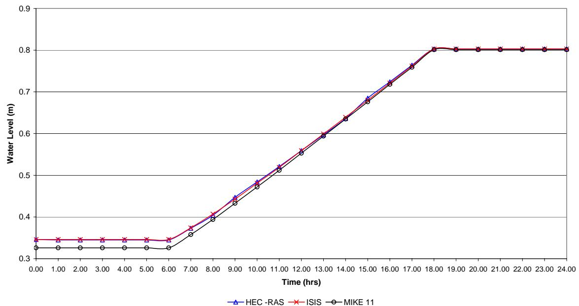
**Graph 2 - Test D Part 2 (Unsteady): Water Levels Upstream of Broad Crested Weir**
