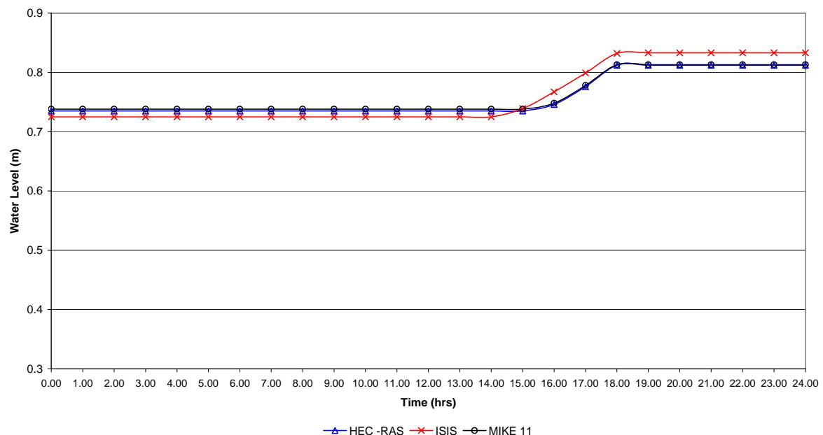
**Graph 3 - Test D Part 2 (Unsteady): Water Levels Downstream of Crump Weir
