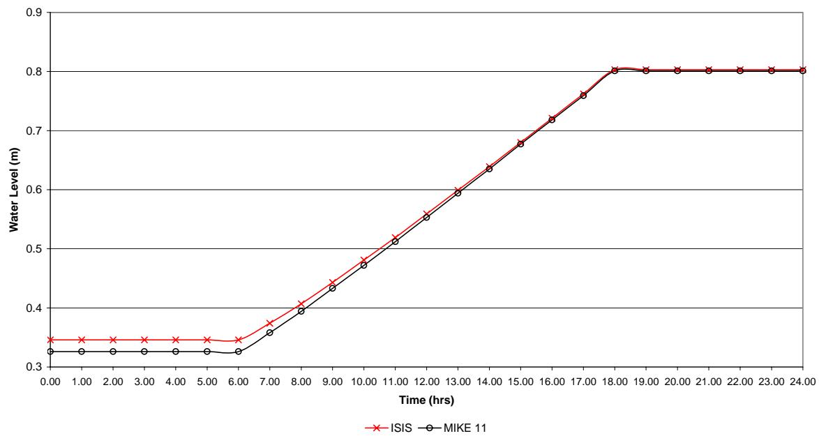
**Graph 4 - Test D Part 2 (Unsteady): Water Levels Upstream of Crump Weir
