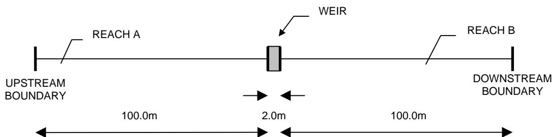
Between Reaches A and B there is a weir. For Part 1 of the test this is a Broad Crested and for Part 2 it is a Crump weir. The parameters defining the weirs are given in Tables 2.1 and 2.2 respectively.
