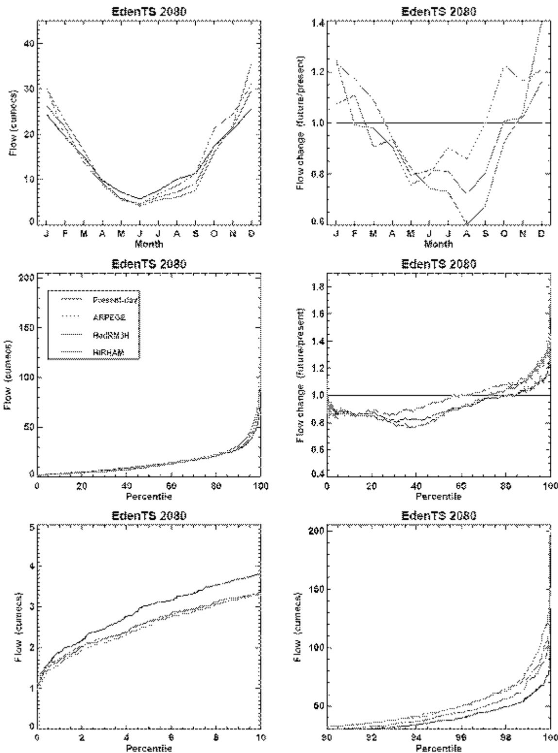
**Figure A1-3a.** Present-day and future flows for the Eden at Temple Sowerby (cumeecs). Top left: mean annual cycle of flows. Top right: mean annual cycle of flows divided by present-day annual cycle. Other rows: flow percentiles (as per previous plot). The present-day flows are black, while the future data are green (ARPEGE), brown (HadRM3H) and pink (HIRHAM).
