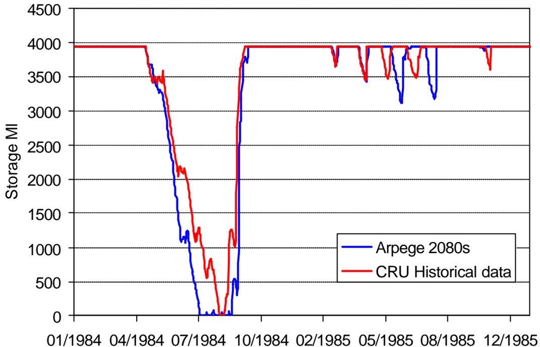
With reservoir yields reduced, the drawdown of Ennerdale Water is marginally later under the ARPEGE scenarios (Figure 5.8a). If the resource was used to meet the demand equal to the current yield, the resource would be drawn down more quickly and the source would fail for a longer period during the WHD year (Figure 5.8b). Lower lake levels would also persist for longer periods. Note that actual abstraction rates from Ennerdale are significantly lower than the yield of the source.
