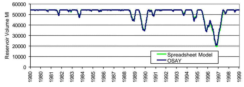
**Figure A2-1: Comparison of spreadsheet model to OSAY outputs for Grafham reservoir (OSAY yield 285 MI/d, spreadsheet model yield 290 MI/d)**
