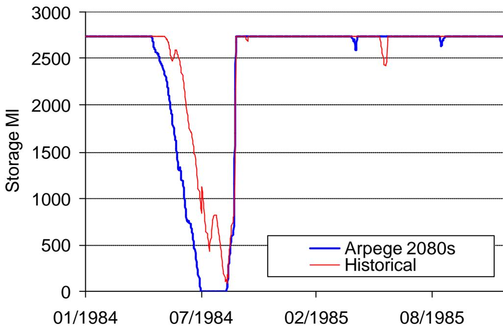
**Figure 5.10: Percentile plot of net storage for Crummock – historical CRU time series compared to ARPEGE 2080s (for run equivalent to Figure 5.9b)**
