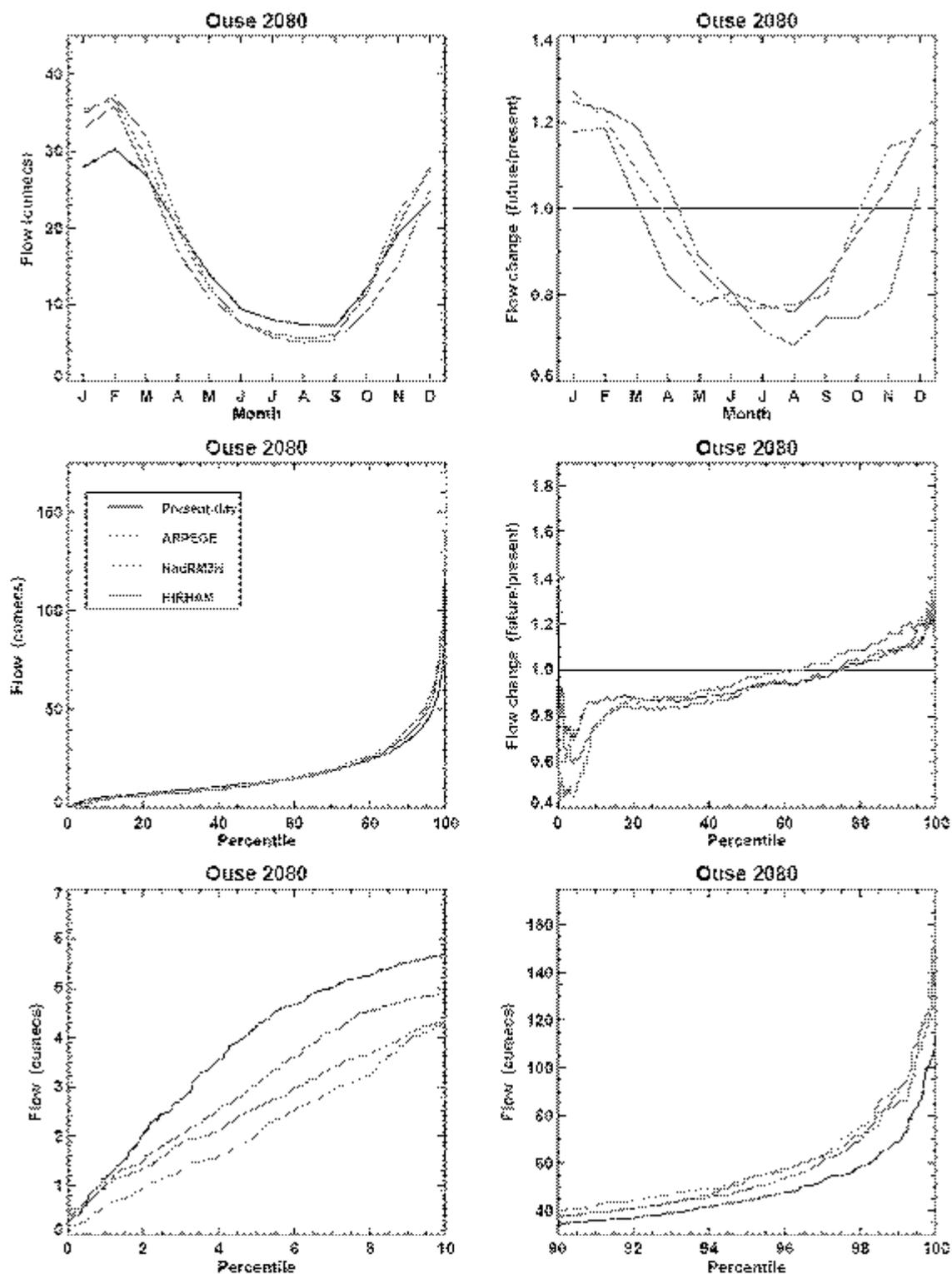
**Figure A1-2a.** Present-day and future flows for the Ely Ouse at Denver Sluice (cumeecs). Top left: mean annual cycle of flows. Top right: mean annual cycle of flows divided by present-day annual cycle. Other rows: changes in percentiles (with 5<sup>th</sup> percentile as a low flow equal to Q95). The present-day flows are black, while the future data are green (ARPEGE), brown (HadRM3H) and pink (HIRHAM).
