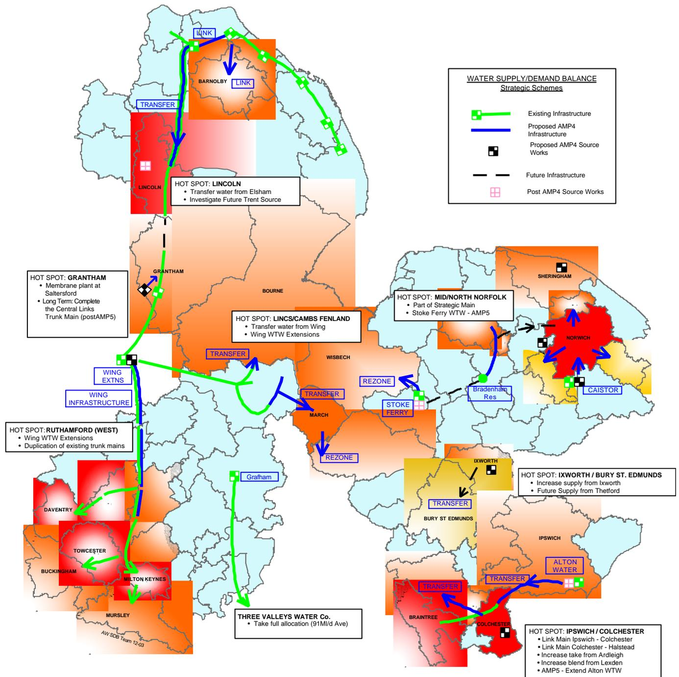
**Figure 4,1: Map showing Strategic Water Supply Schemes in Anglian Water's supply area (Source: Anglian Water Services Water Resources Plan Digest, 2003). <http://www.anglianwater.co.uk/assets/WRP04final.pdf> )**
