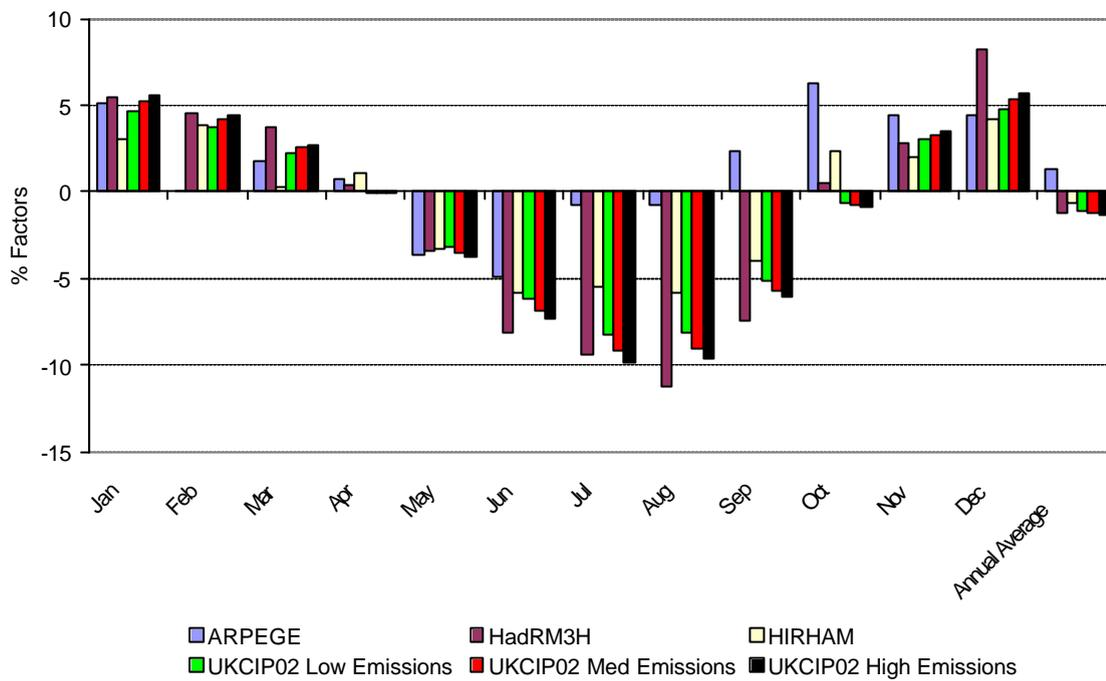
**Figure 5.5: Comparison of monthly PET factors for the 2020s, three RCMs for the River Eden and UKCIP02 data for the Eden CAMS**
