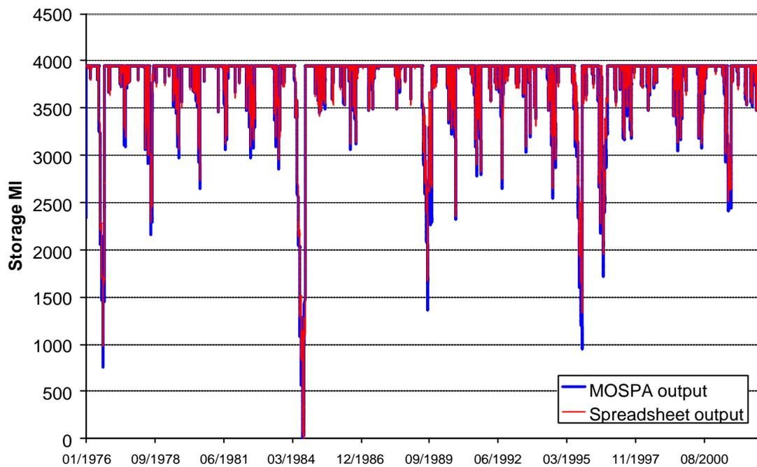
**Figure A2-2: Comparison of spreadsheet model to MOSPA outputs for Ennerdale. (Yield is 55.23 MI/d for both models)**
