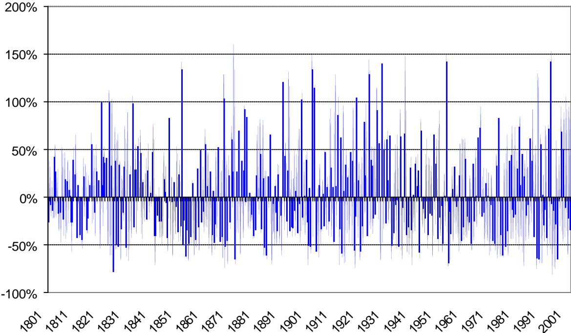
**Figure 3.3: Characteristics of historical periods compared to the 1961-90 period for the Ouse at Denver Sluice: (a) monthly differences in flow; (b) differences in average flow. (For each plot the data describes 30-year blocks centred on the listed decade)**
