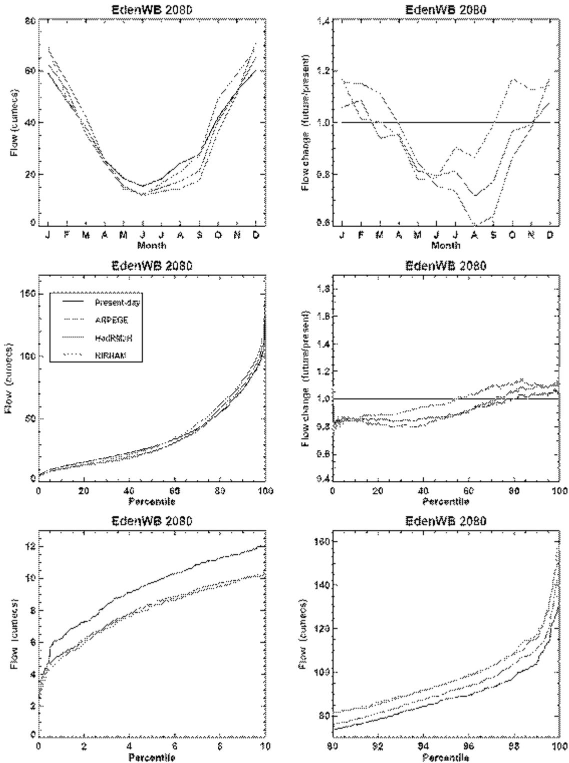
**Figure A1-4a.** Present-day and future flows for the Eden at Warwick Bridge (cumecs). Top left: mean annual cycle of flows. Top right: mean annual cycle of flows divided by present-day annual cycle. Other rows: flow percentiles (as per previous plot). The present-day flows are black, while the future data are green (ARPEGE), brown (HadRM3H) and pink (HIRHAM).
