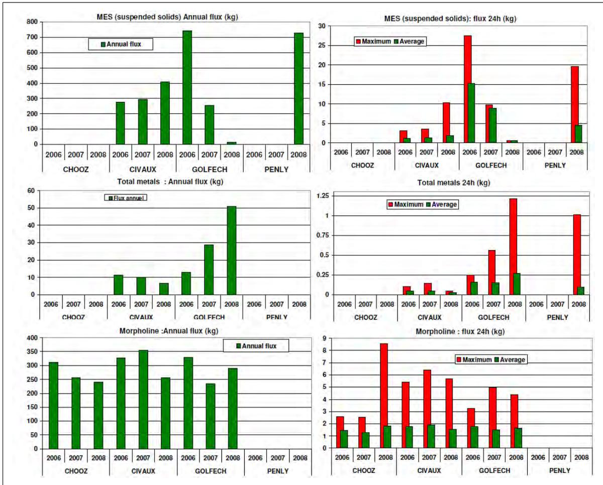
**Figure A6.3** Suspended solids, metals and morpholine associated with liquid radioactive effluents from the nuclear island and turbine hall discharge (KER-SEK)
