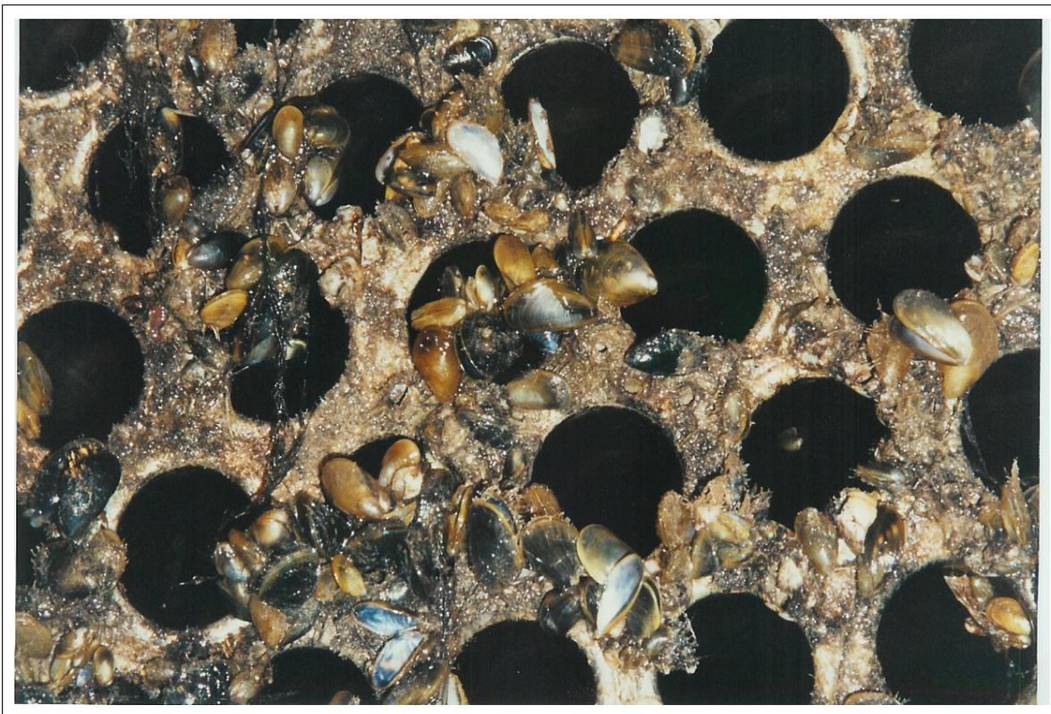
**Figure 4.4 Mussel infestation at the entry to the cooling tubes in the main condenser (By permission of KEMA)**
