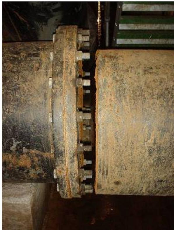
**Figure 5-12 Fractured compensation pipework (above) and fractured 30-inch (769-mm) diameter scour pipe (below) adjacent to bolted flanges (after Hughes *et al.*, 2004)**
