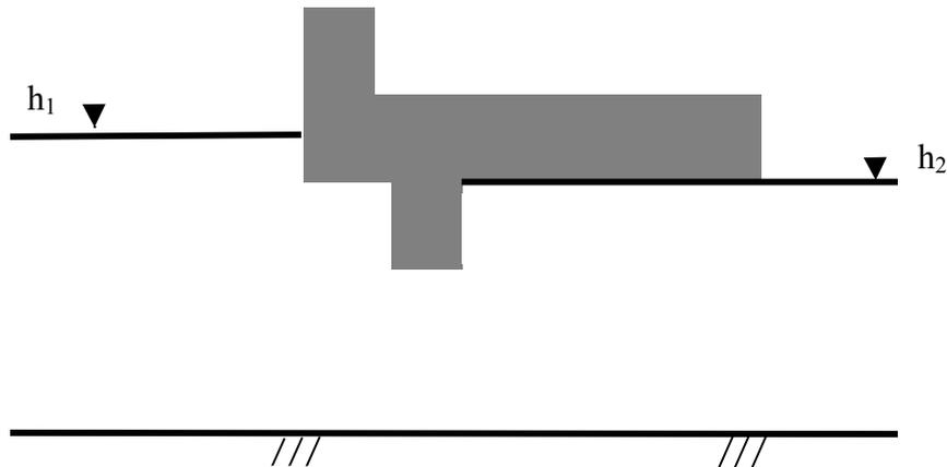
**Figure 3.5 Submerged flow**
