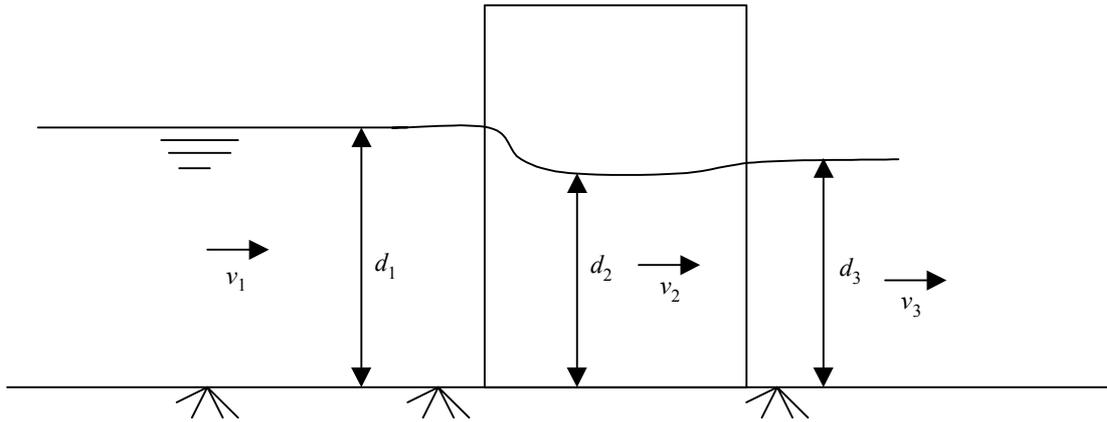
**Figure 3.1 Elevation view of channel constriction (energy analysis)**
