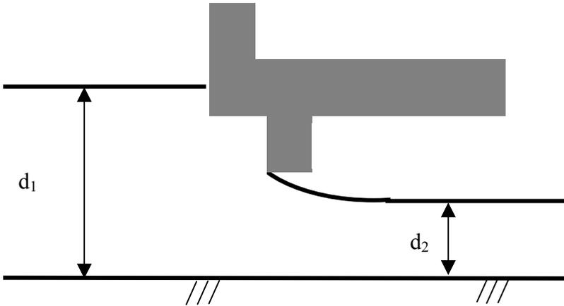
Figure 3.4 Orifice flow
