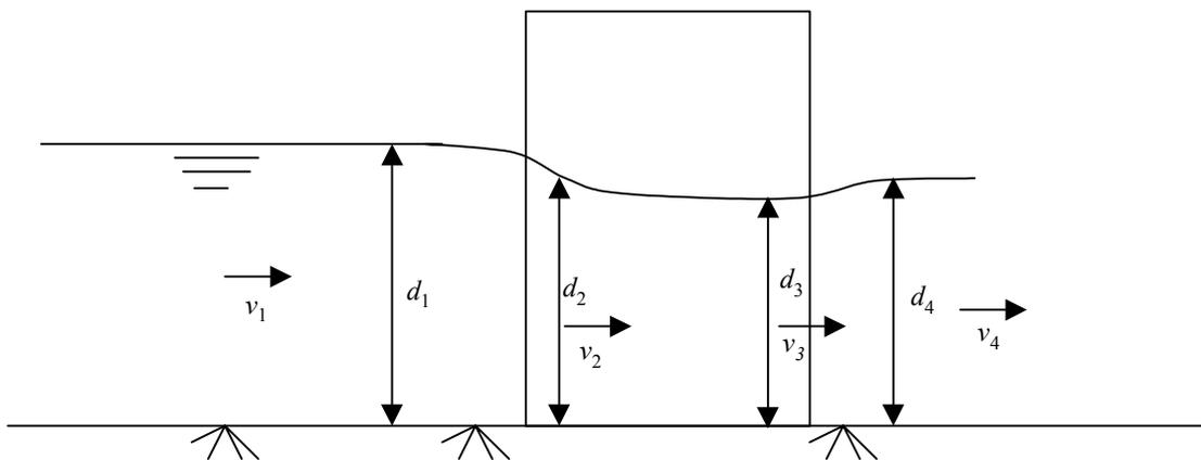
**Figure 3.2 Elevation view of channel constriction (momentum analysis)**
