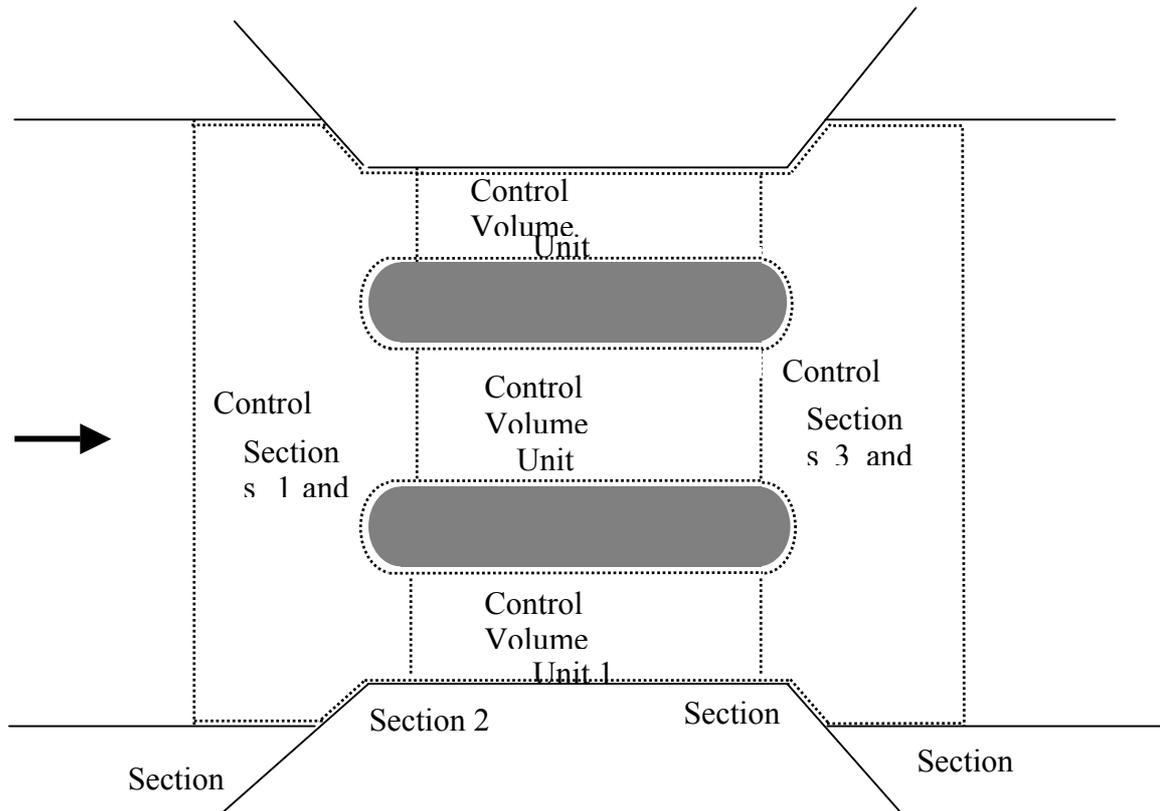
**Figure 3.3 Plan view of channel constriction (momentum analysis)**
