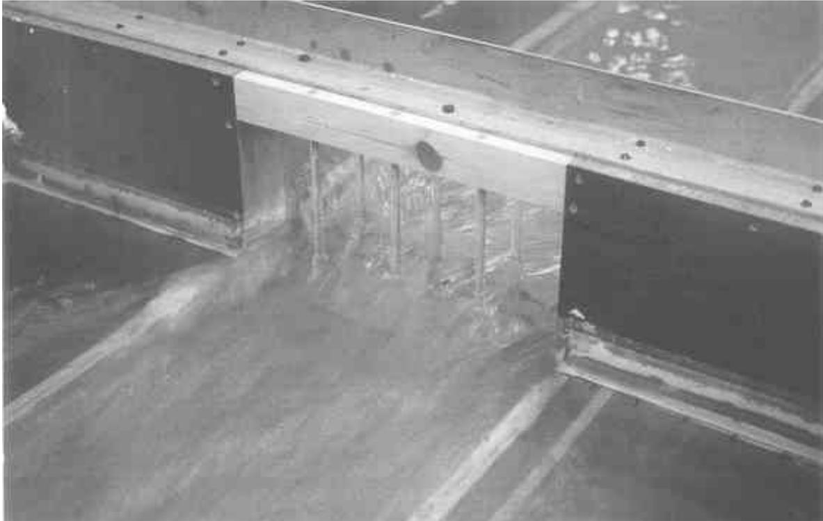
**Figure 9: Observed flow through a model bridge with circular piers in a compound channel (Atabay & Knight, 2002).**
