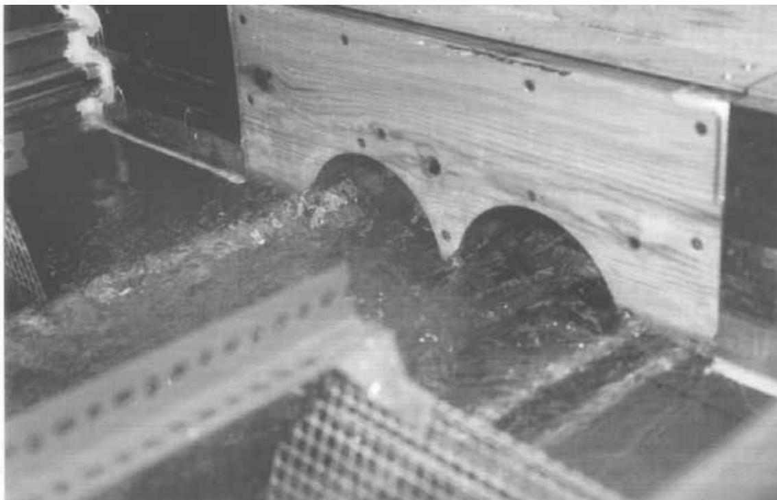
**Figure 12: Observed flow through a model twin arch bridge in a compound channel, viewed from downstream (Atabay & Knight, 2002)**
