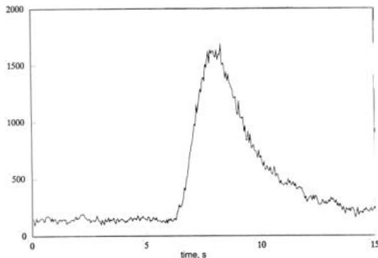
**Figure 15 - Residence Time Distribution of 0.1s Pulse of He Injected Into Secondary Front Air**
