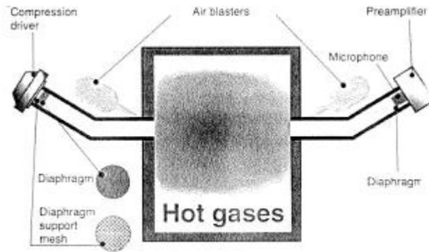
**Fig 2a - Schematic Illustration of a Acoustic Pyrometer System**
