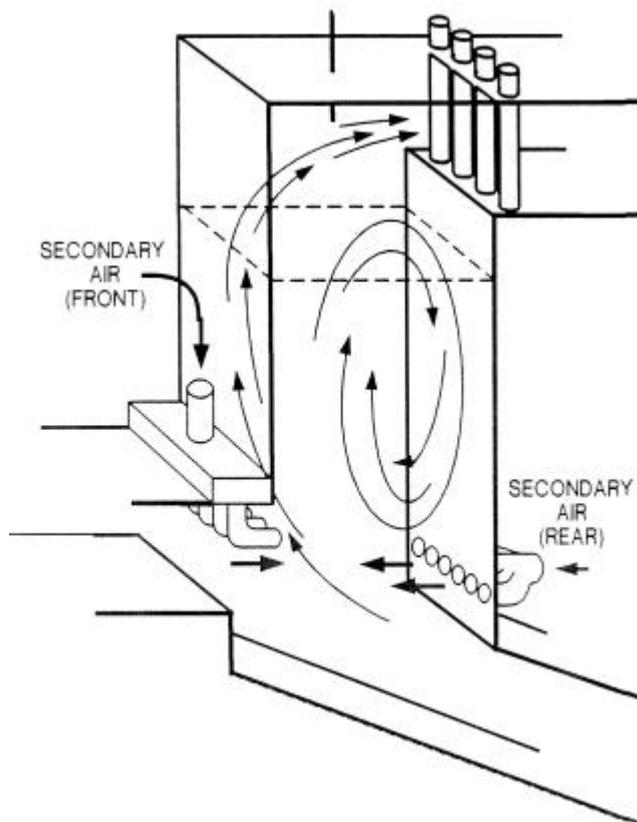
**Fig 7 - Likely Flow Pattern Showing Channelling and Re-Circulation**
