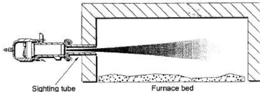
**Fig 4 - Infrared Pyrometer**
