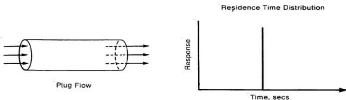
Figure 1a - No Mixing (Plug Flow Model)
