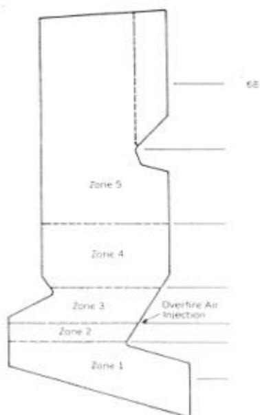
**Fig 9 - Typical Zones of a Combustion Chamber (Energy from Waste Incinerator)**
