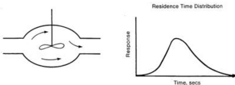
Figure 1c - Real Situation (Partially Stirred Reactor)
