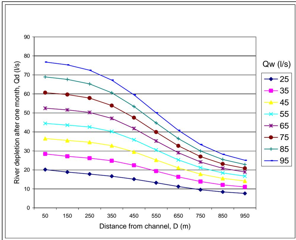
**Figure 3.4 – Depletion of river flow due to pumping a well at a variety of abstraction rates and a variety of distances from the river**
