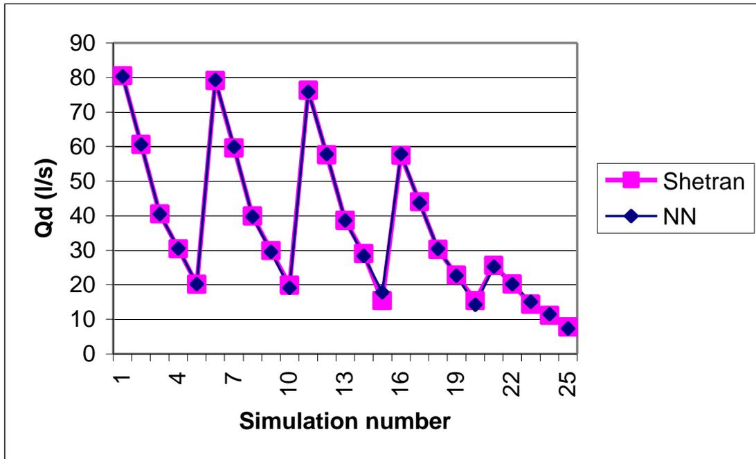
**Figure 3.3 – Excellent correspondence between neural network (NN) and SHETRAN output following the training of the former (root mean-squared error = 1.7%)**
