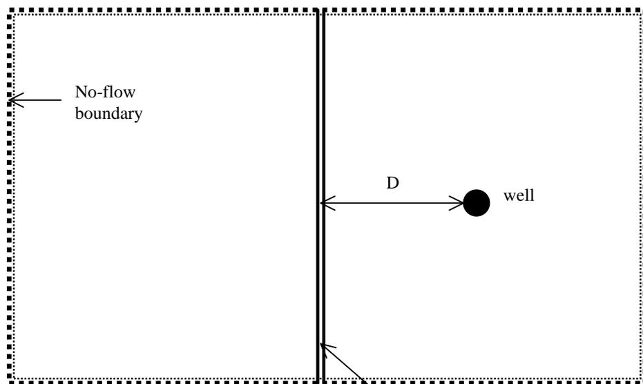
Figure 3.1 – Map of idealised stream-aquifer system analysed in this case study.
