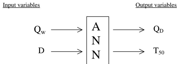
**Figure 3.2 – Schematic sketch of the artificial neural network used in this case study**
