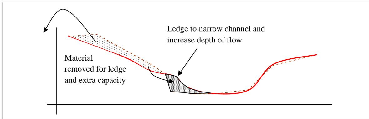
**Figure 6.6 Re-profiling of a cross-section on the River Rhee**
