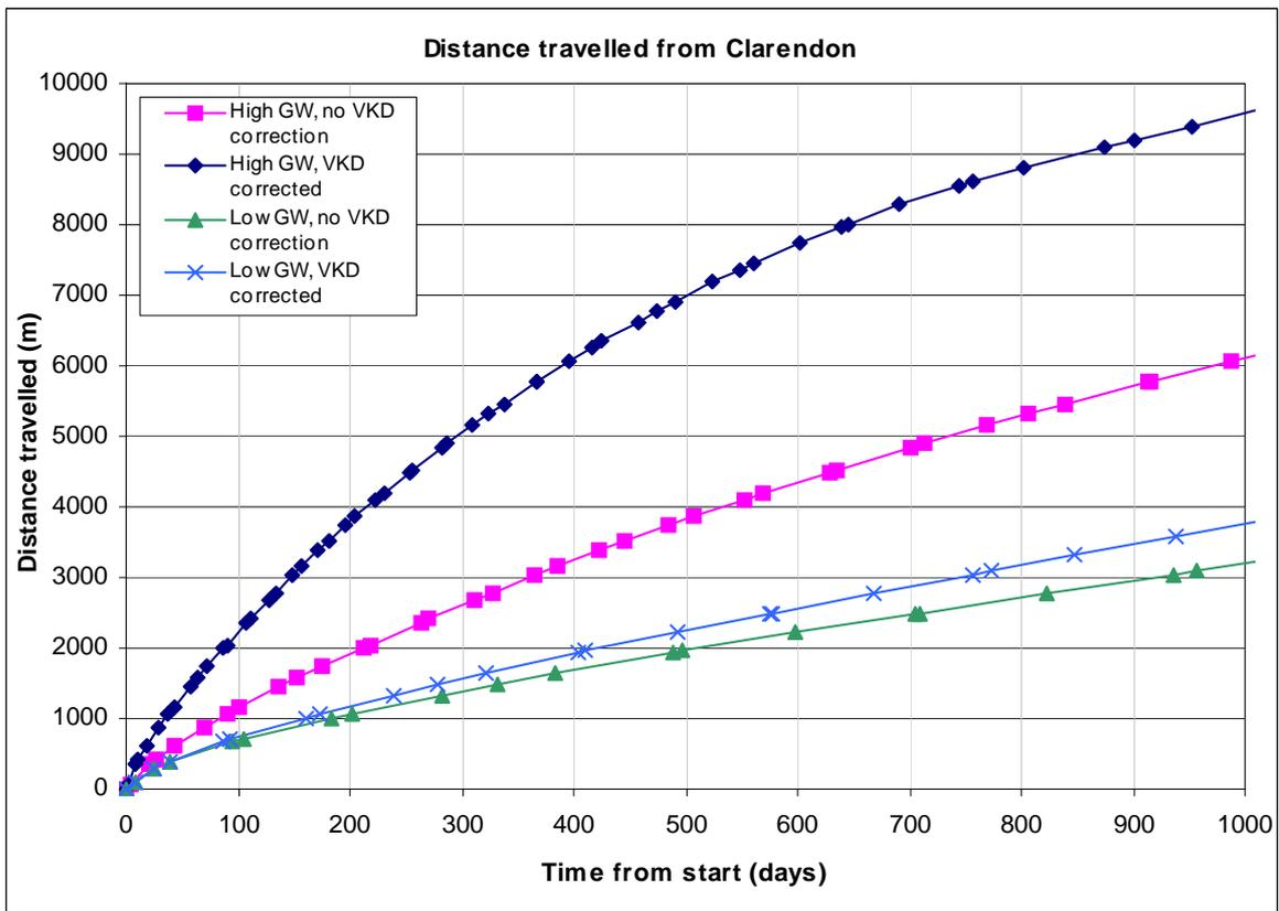
Figure 3.5 Steady state backwards tracking from Clarendon Park abstraction with VKD correction
