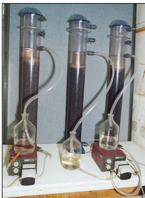
Plate 11 Columns filled with bottom ash
