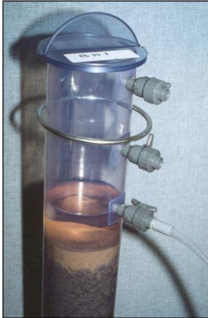
Plate 12 Column test, detail
