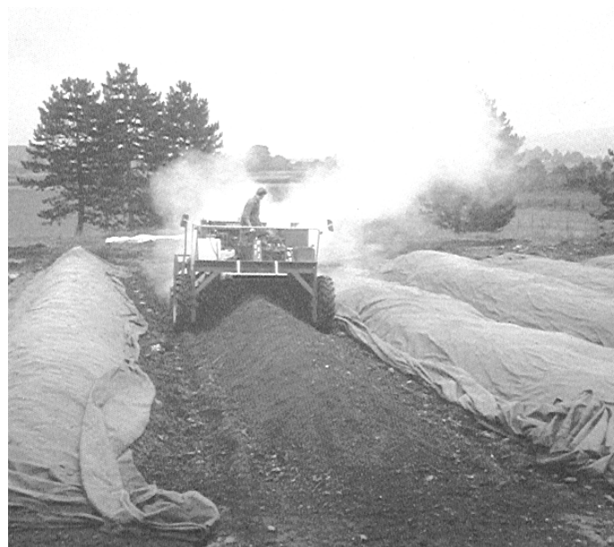
Figure 8-1: Sandberger system with covered and uncovered windrows
