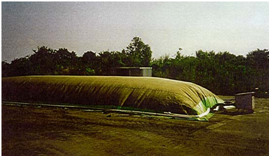
Figure 8-2: Gore-Tex covered aerated static pile
