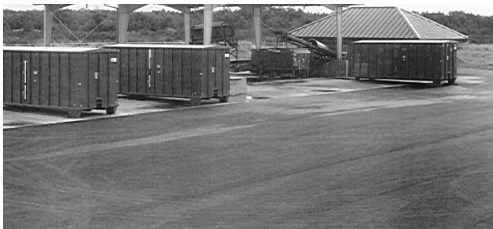
Figure 10-43: Green Mountain Technology CompTainer batch tunnel (3 units)
