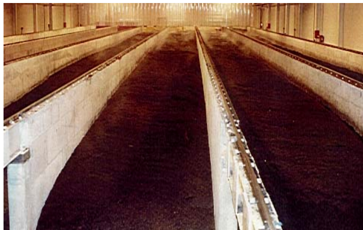
Figure 10-13: Longwood Manufacturing- Agitated bays filled with compost
