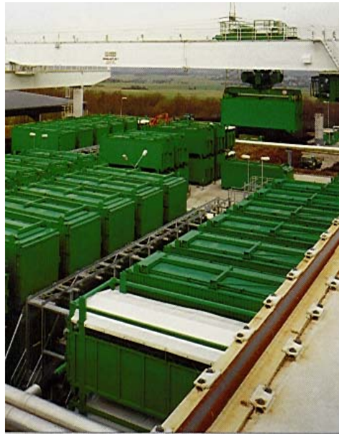
Figure 10-44: Lurgi containers - showing containers stacked two-high
