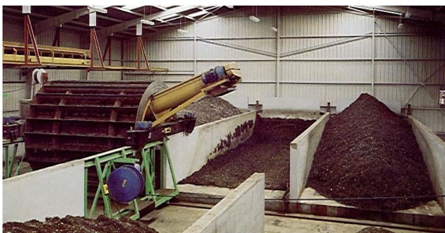
Figure 10-24: OTV composting bays
