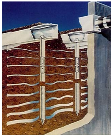
Figure 10-2: American Bio Tech - air lances providing lateral movement of air
