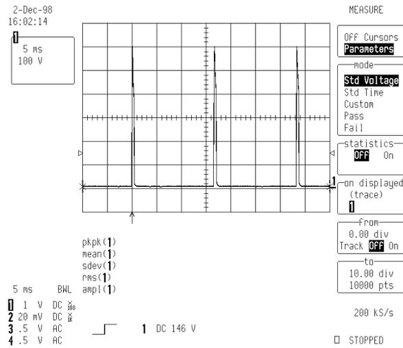
**Figure A1.5** Gated burst waveform.
