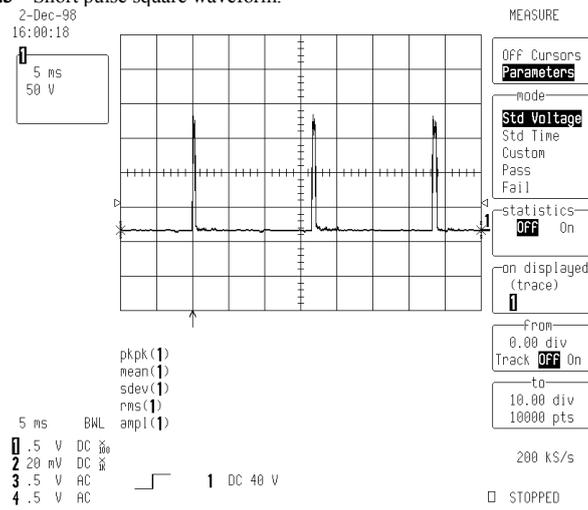
**Figure A1.4** Short pulse square waveform - high voltage.
