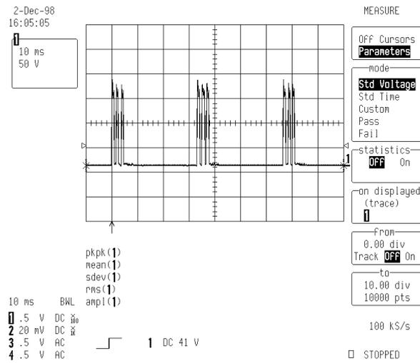
**Figure A1.6** Gated burst - high voltage waveform.
