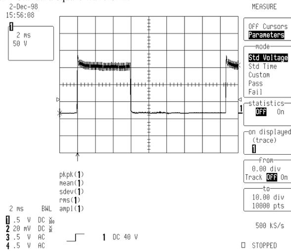
**Figure A1.3** Short pulse square waveform.
