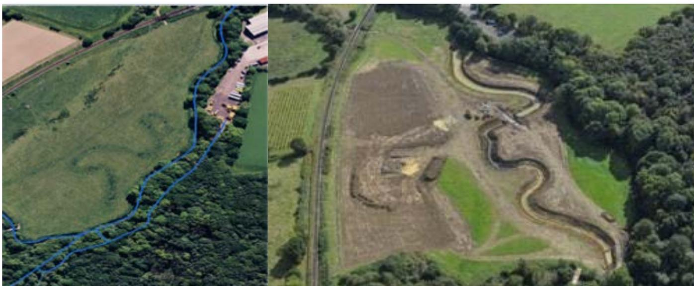
**LEFT: Before MORPH - the river (blue lines) had been straightened, widened and given steep banks for navigation in the past. The old meander (wiggle) in the river is visible in the field. RIGHT: Photo taken during the works. The river has been re-meandered and brought back through the field. This creates different flows and habitats which will bring more wildlife to the river and slow the movement of water through the river.**
