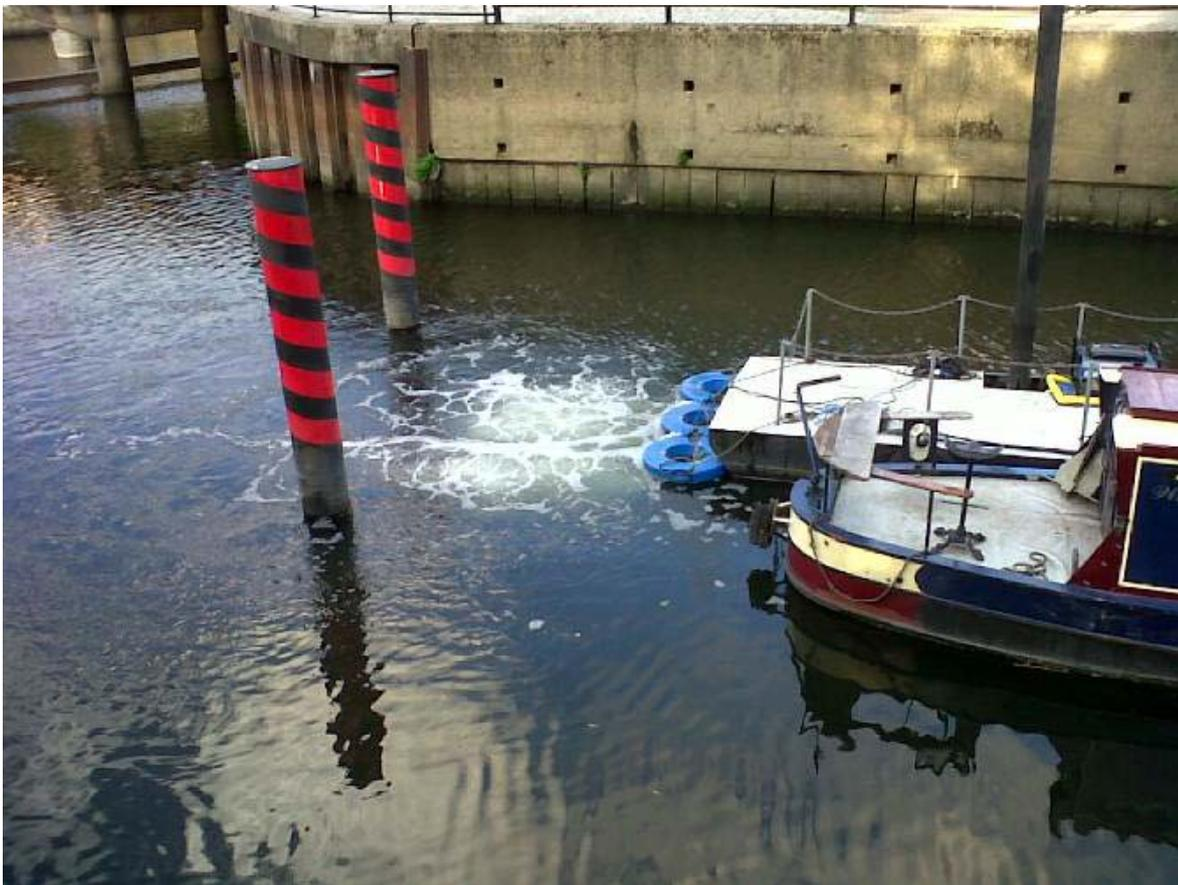
**Aeration equipment was used to boost oxygen levels on the River Lee**
