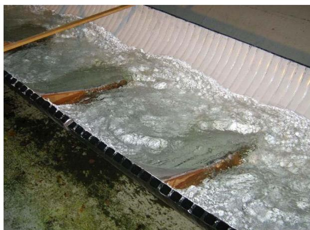
**Culvert with baffles to improve eel passage**
