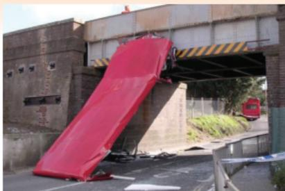
*The roof of a double deck bus removed in a bridge strike*
