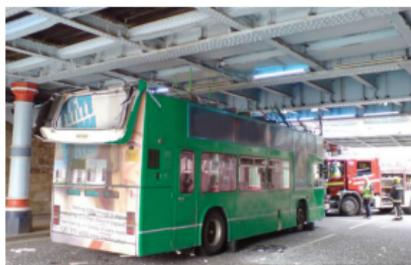
*Double deck bus without a roof under a bridge*
