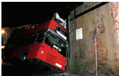
*Bus resting against the bridge abutment following a bridge strike at a skew bridge*
