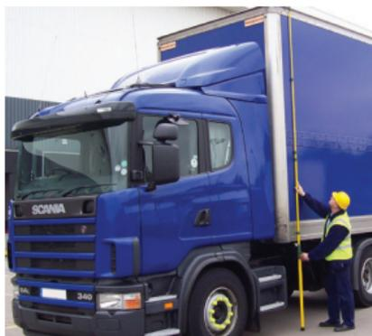
*Always check the maximum height of your vehicle, its load and equipment*
