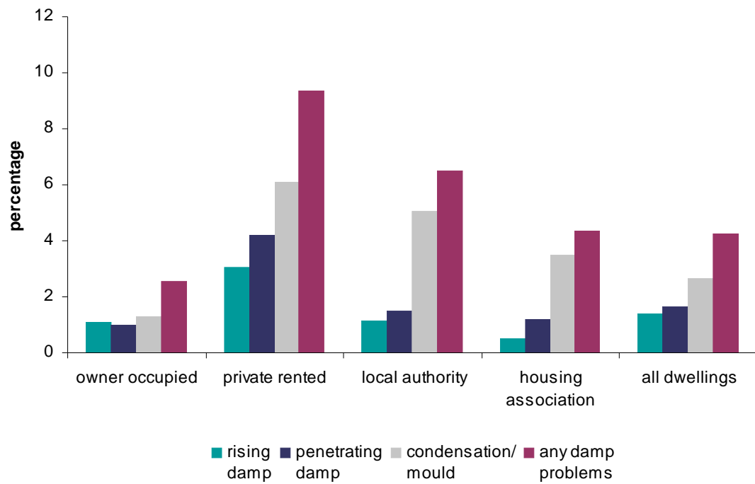
Figure 18: Damp problems, by tenure, 2012
