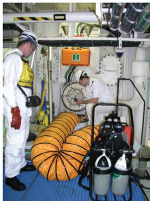
**17.5.6** Where necessary pumping operations or cargo movements should be suspended when entry is being made into a dangerous space.
