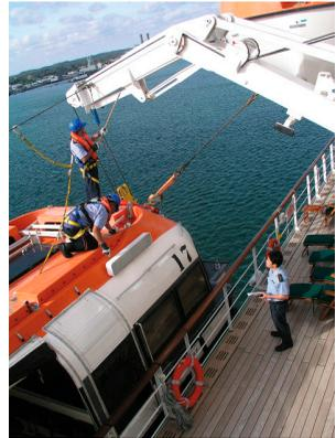
**15.2.6** Other than emergency situations personnel should not work overside whilst the vessel is underway. If such work has to be undertaken lifeboats or rescue boats should be ready for immediate use. Any such work should be closely monitored/watched by a responsible person.
