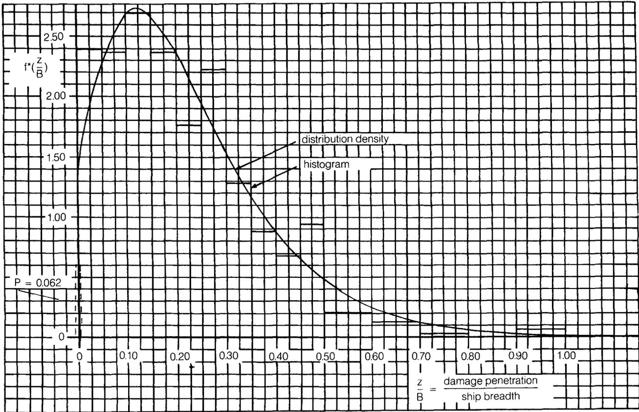
FIGURE 15 - DISTRIBUTION DENSITY OF NON-DIMENSIONAL DAMAGE PENETRATION
