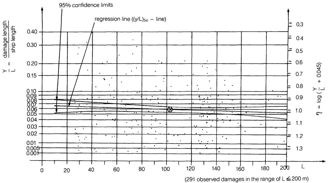
FIGURE 9 - REGRESSION OF NON-DIMENSIONAL DAMAGE LENGTH ON SHIP LENGTH
