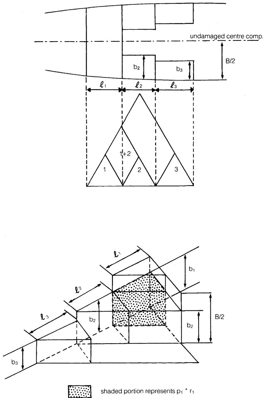
$$\text{The } p \text{- factor for comp. } 1 + 2 : p = p_{12} * r_{12} - p_1 * r_1 - p_2 * r_2$$
