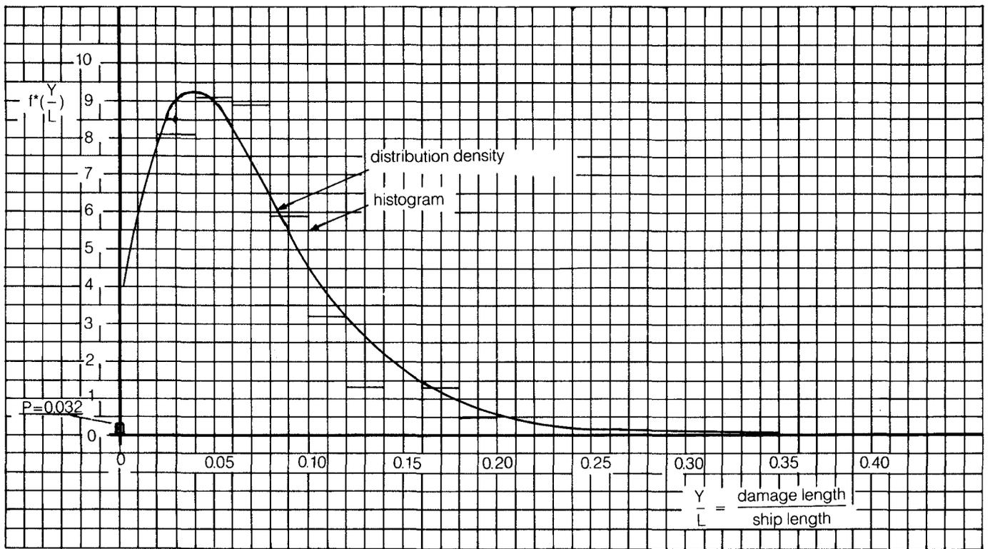
FIGURE 8 - DISTRIBUTION DENSITY OF NON-DIMENSIONAL DAMAGE LENGTH
