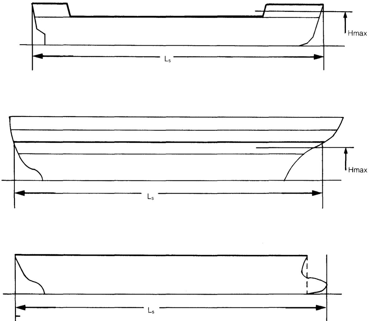
a deck, or decks, which limit the highest vertical extent of flooding
