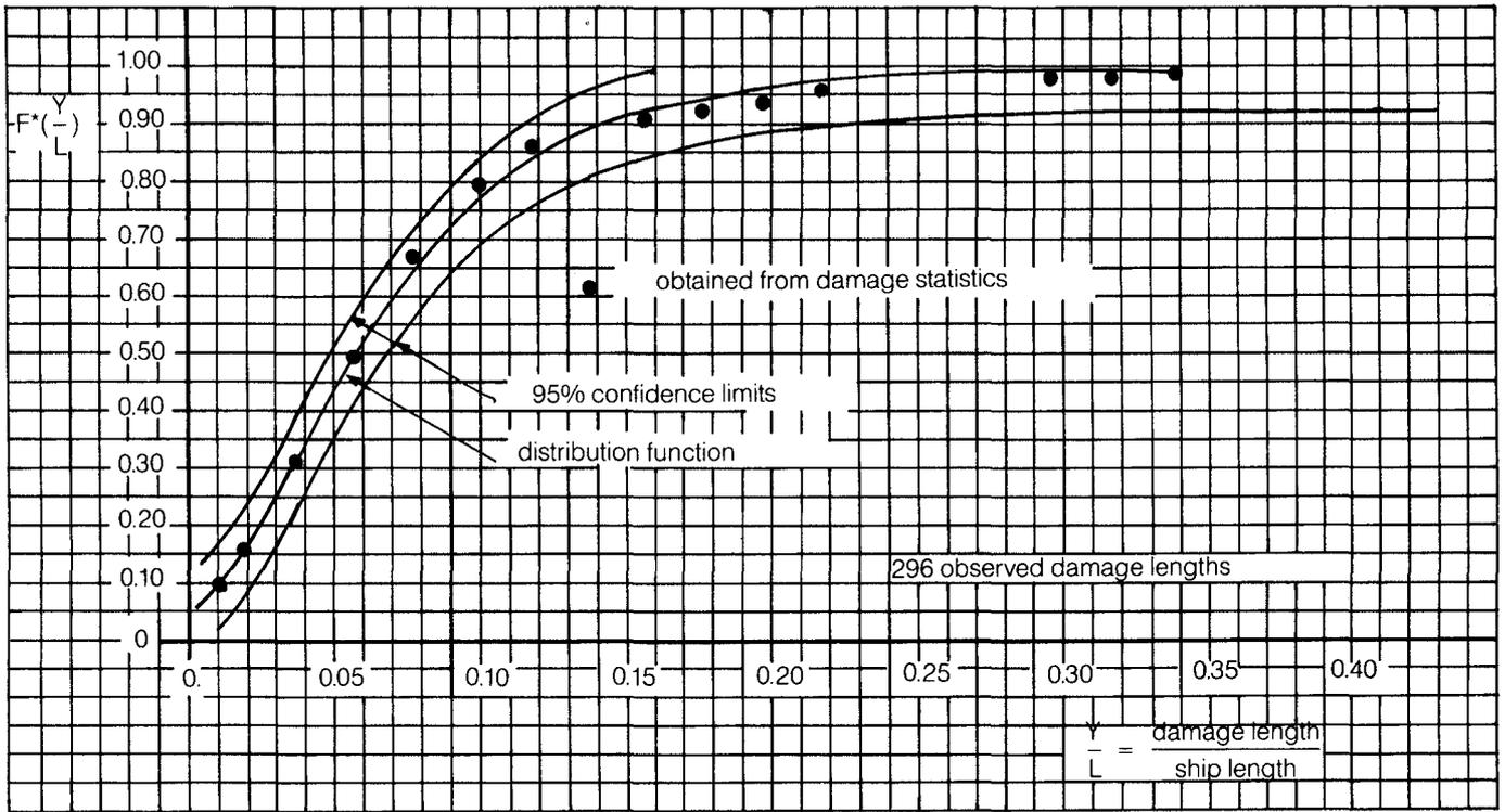
FIGURE 7 - DISTRIBUTION FUNCTION OF NON-DIMENSIONAL DAMAGE LENGTH
