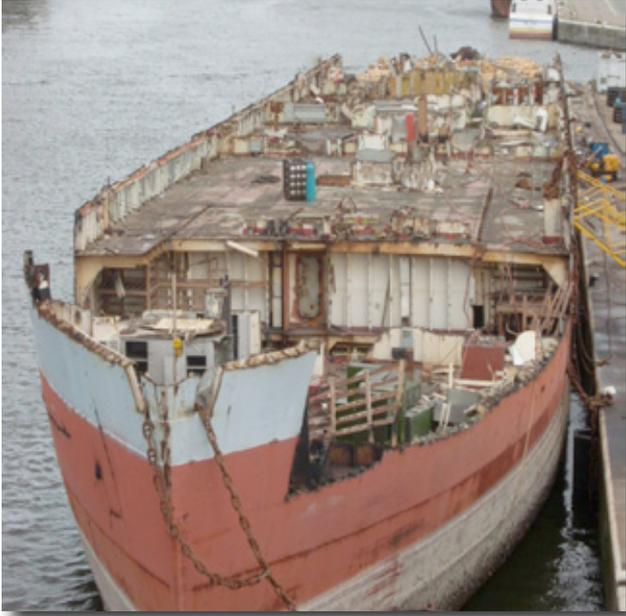
Deck 3 prior to being cut & removed
