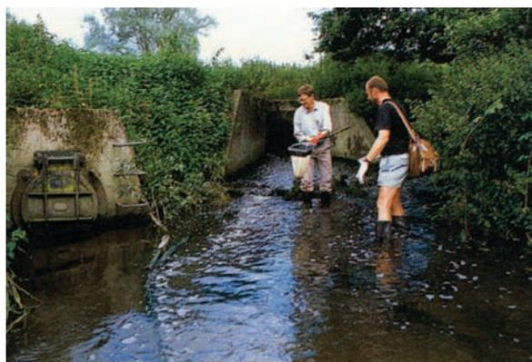
Survey of the impacts of a sewage discharge in a small stream.
