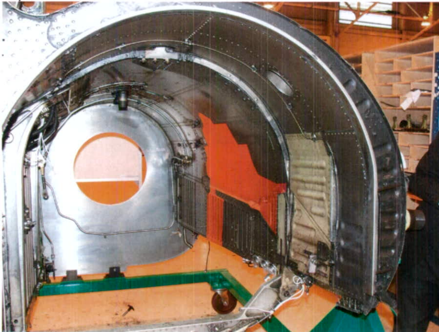
Figure 15 - Representative area of right firewall recovered
