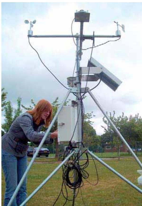
Tracking the risk of bluetongue: a portable automatic weather station will be deployed to areas that become infected, which will ensure that the weather conditions in the close vicinity of any infected animals are well-defined
